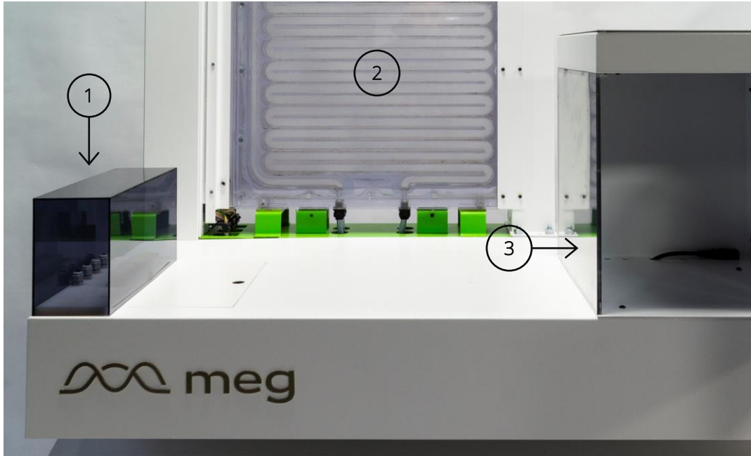
① Sensors ② Hydraulic Panel ③ Microalgae inoculation light box
