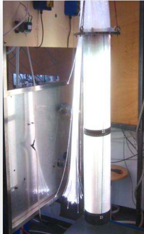
DiCoFluV 1 volumetrically illuminated PBR (courtesy of Institut Pascal – UCA - France)
