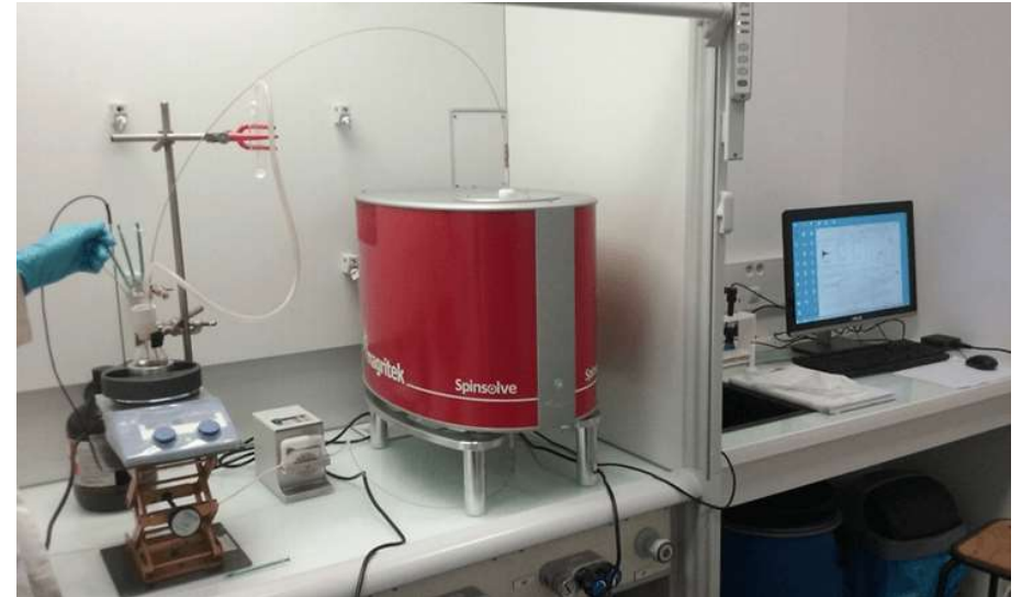
Benchtop NMR used for reaction monitoring
