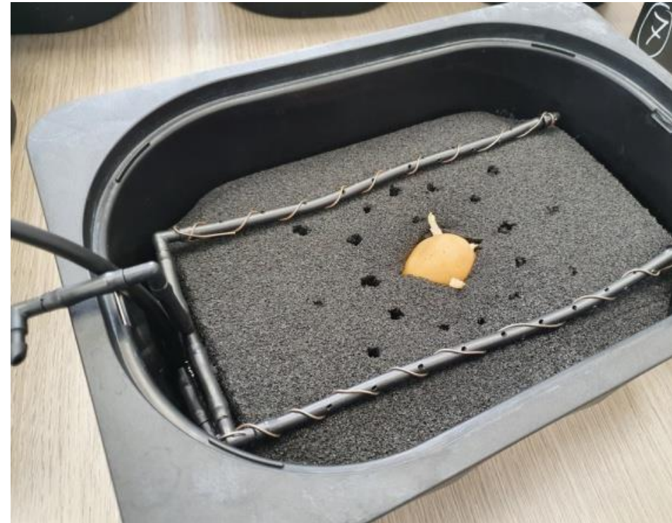
Perforated pipes (36 holes)
