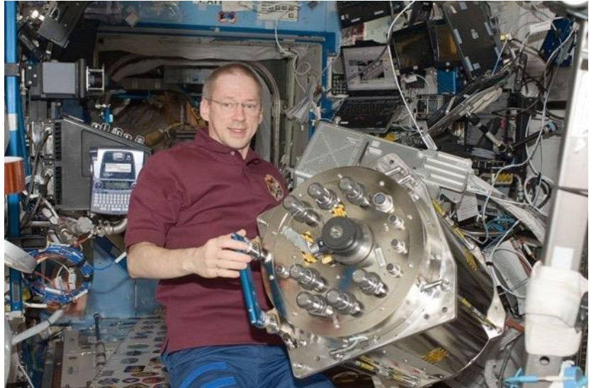
Belgian astronaut Frank De Winne repairing the Urine Processor Assembly (UPA)
