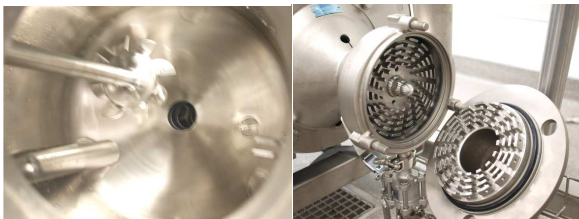
Figure 4: View of tank (left) and shear pump head (right) after cleaning.
