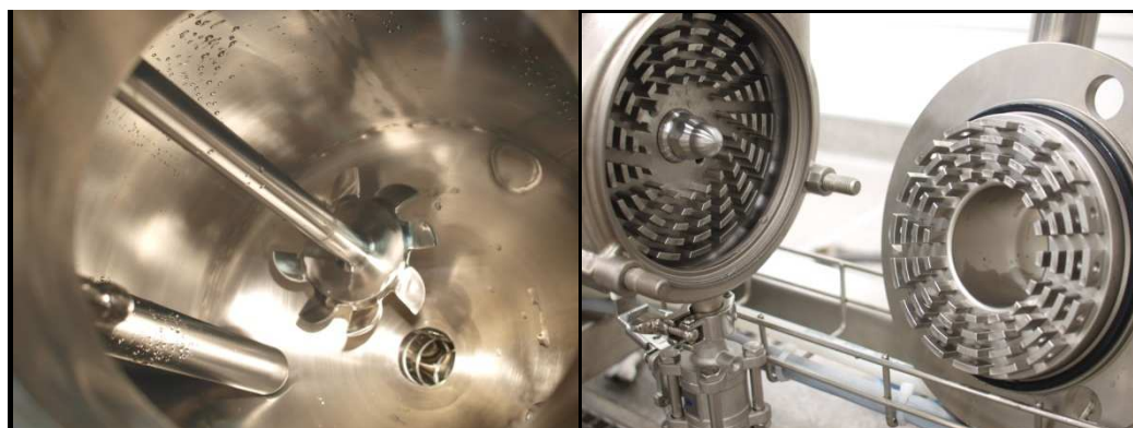
Figure 5: View of tank (left), and shear pump head (right) after complete cleaning cycle.
