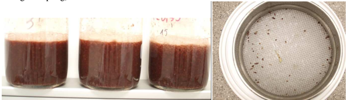
Figure 2: View of waste mixture samples (left) and remaining material on 2 mm mesh sieve (right).
