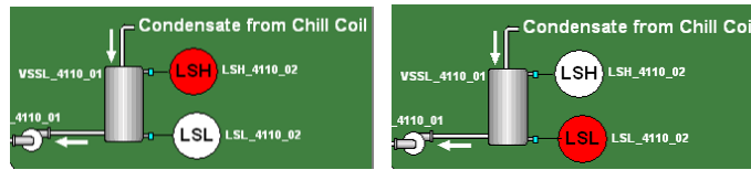
Figure 23: High and Low level alarm of the condensate tank
