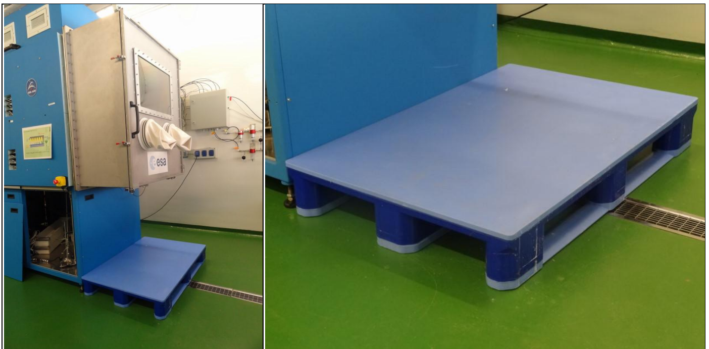
Figure 11: Access platform to HPC1 airlocks
