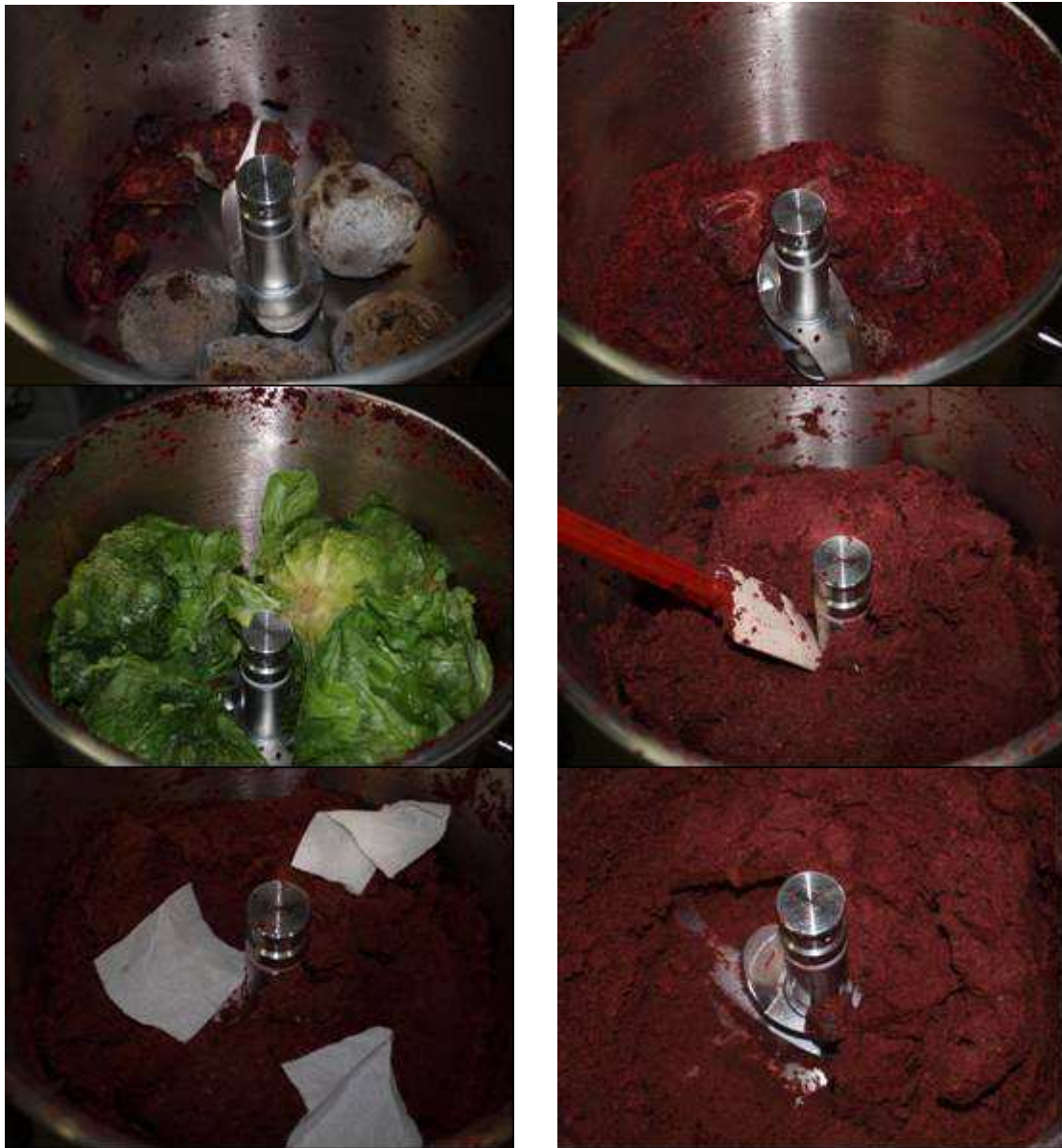
Figure 6. Cutting result (right) after sequential addition of red beet, lettuce and toilet paper (left) to the same batch.
