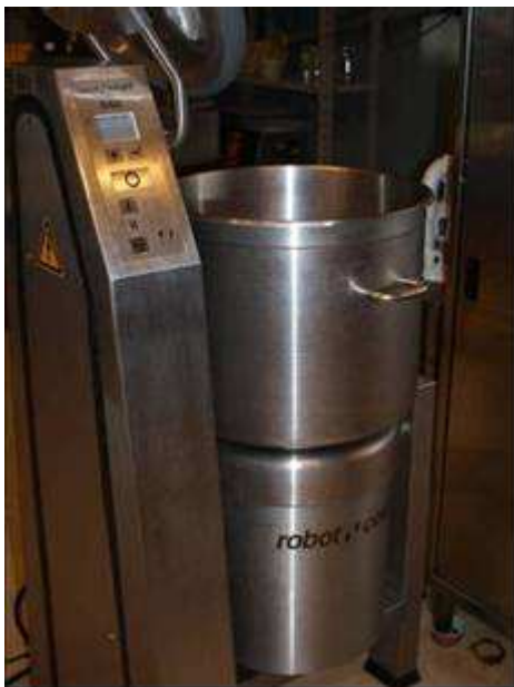
Figure 5. Picture of vertical cutter (left), and close-up of milled edges (right).
