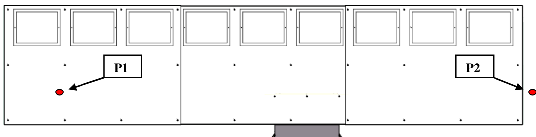
Figure 6 Pressure probes in the plenum of the chamber
