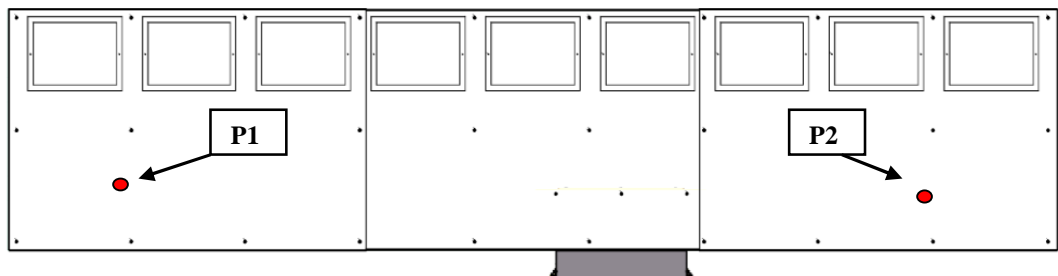
Figure 4 Pressure probes in the plenum of the chamber
