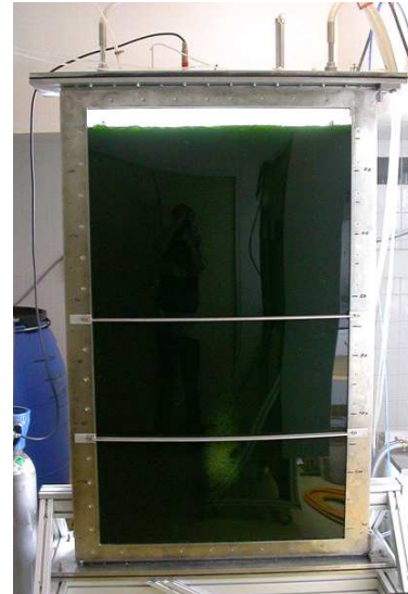
Airlift PBR (Pilote-scale PBR)
