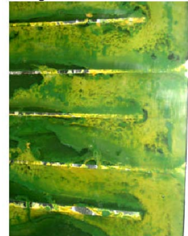
Sedimentation/Adhesion of algae onto reactor walls
