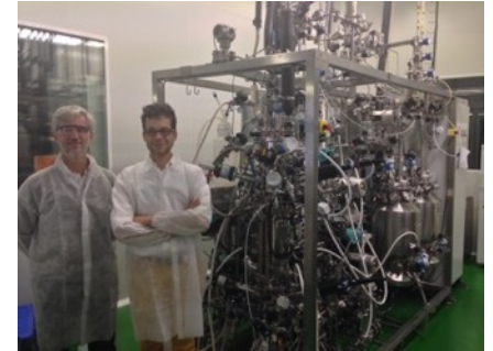
Nitrification bioreactor at the MELiSSA pilot plant
