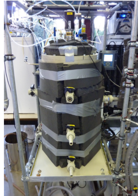
Anaerobic liquefaction sub-system
