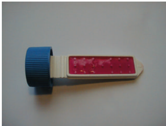
Figure 8: Standard sterility test (Merck) for the detection of micro-organisms in aqueous media
