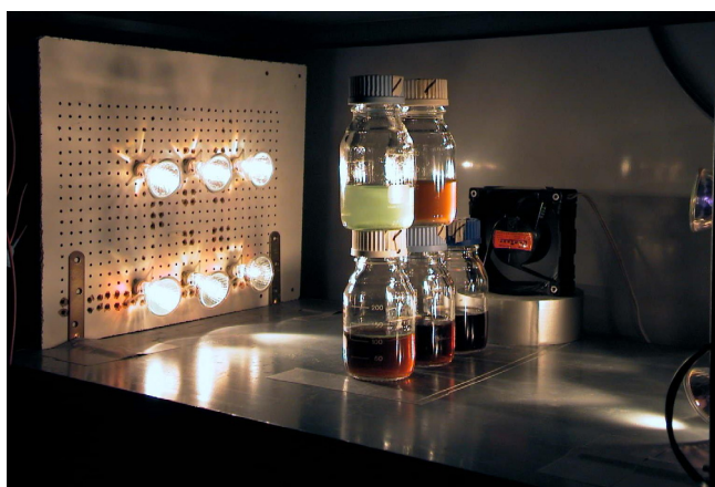
Figure 3.5.- Experimental set-up of the S. platensis and R. rubrum batch-tests.
