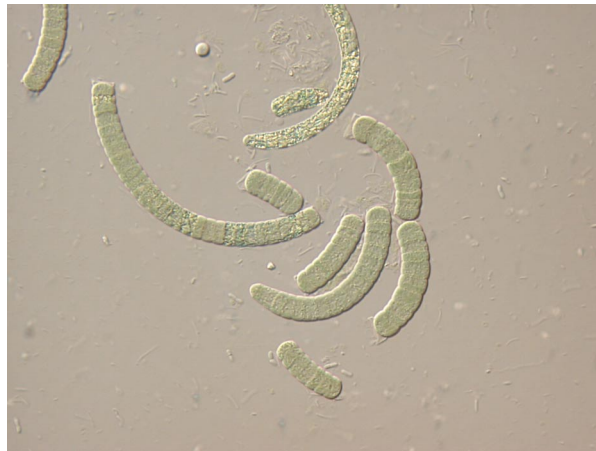
Figure 10. Microscopic view (400 X) of Arthrospira platensis in the concentrated stream of the filtration unit. Filaments fragmentation and dispersed cell inclusions are observed.
