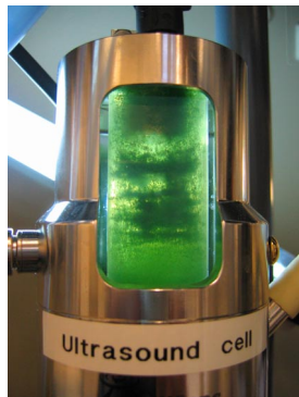
Figure 4: Aggregation of alga cells in the resonance chamber
