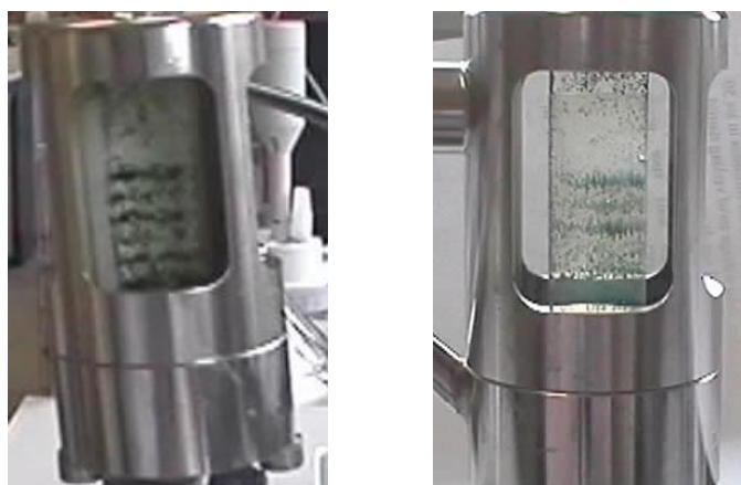
Figure 9. Aggregation of algae cells in the resonance chamber.
