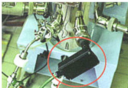
Figure 17: Biomass probe fits as standard 25mm Ingold type port. 19mm top entry is also available.
