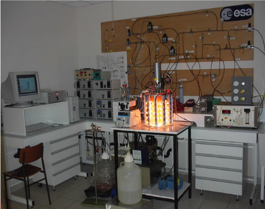
Figure 3 : Experimental system used for the Rs. rubrum photoheterotrophic growth in chemostat mode.
