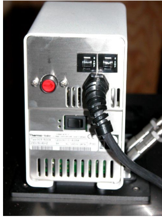
Figure 2. back side of the cooler temperature control
