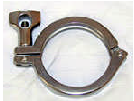
Figure 5: Clamp, which holds two pipe ends together
