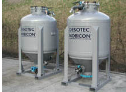
Figure 37: Non-aerated GAC mobile filters
