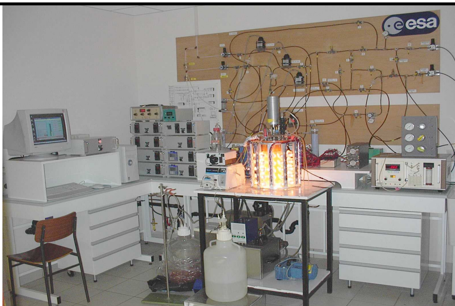
Figure 1: Photograph of the 5 L – working volume cylindrical photobioreactor radially illuminated used in this study in chemostat mode.
