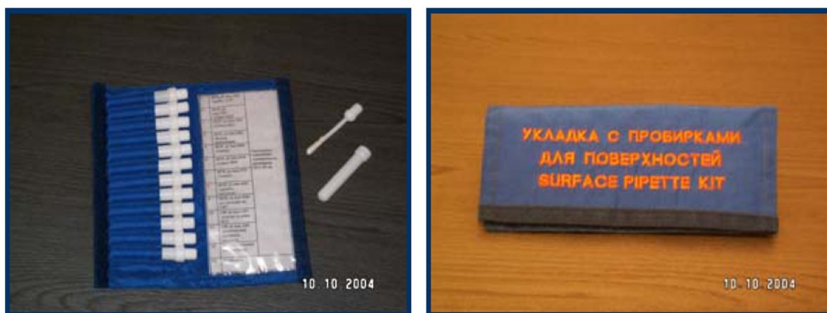
Fig. 2. Surface pipette kit for sampling internal surfaces and structural materials of the ISS.
