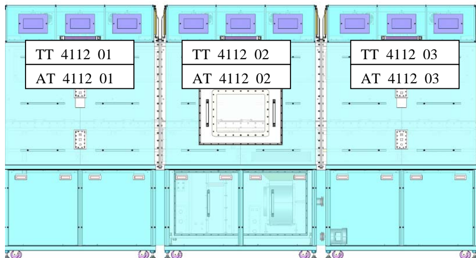
Figure 25 Position of chamber temperature and humidity sensors.
