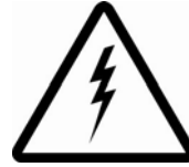
Electrical Shock Hazard Caution or Warning
