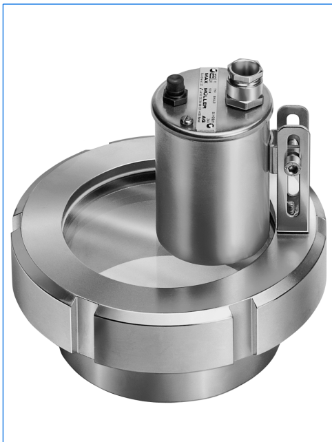
Sightglass light fitting type BKVLR 50 HDSch1, 50 W, 24 V, with built-in momentary push-button "D", mounted with tilting hinge "Sch1" on screwed sight-glass similar to DIN 11581, DN 100, PN 6, for application "view and light through one assembly".
