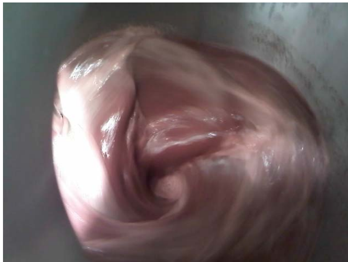
Figure 5: Vortex effect created by the shear pump impulsion of the mixture within the vessel during the milling process.
