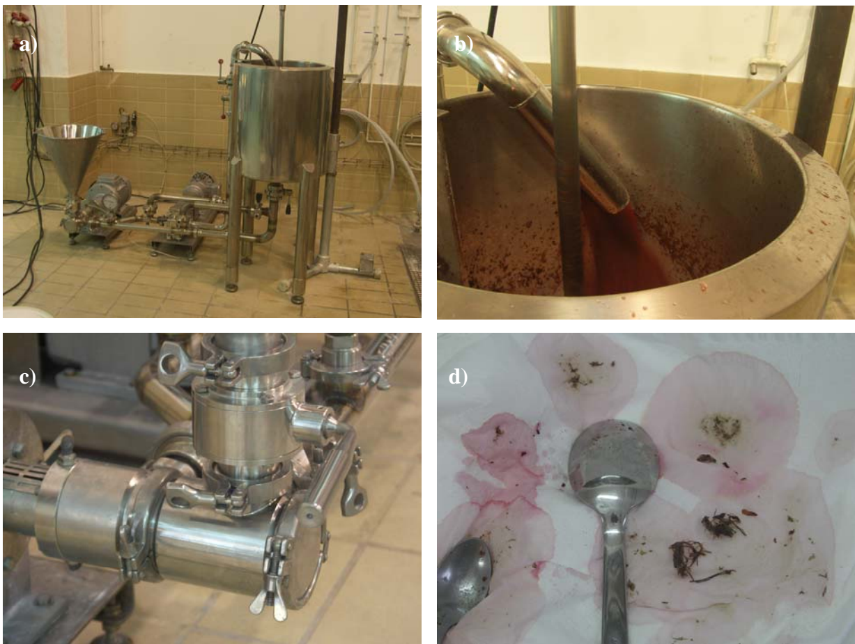
Figure 11. a) VISCOVAK in-line mixer and ancillary equipment (VAK KIMSA Pilot Plant, Barcelona); b) fluid recirculation after passing the mixer; c) details of the mixing head; d) detail of non milled particles
