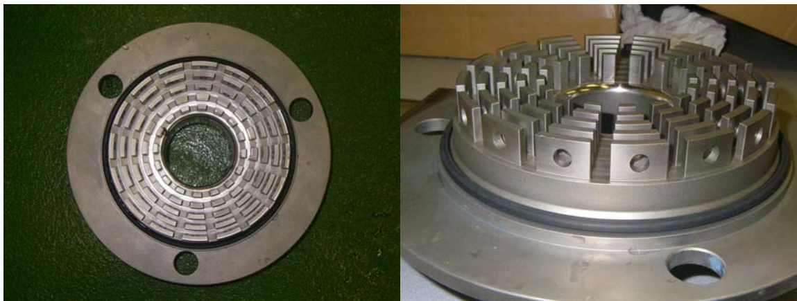
Figure 8. Stator with drilled teeth tested in the FRISTAM shear pump.
