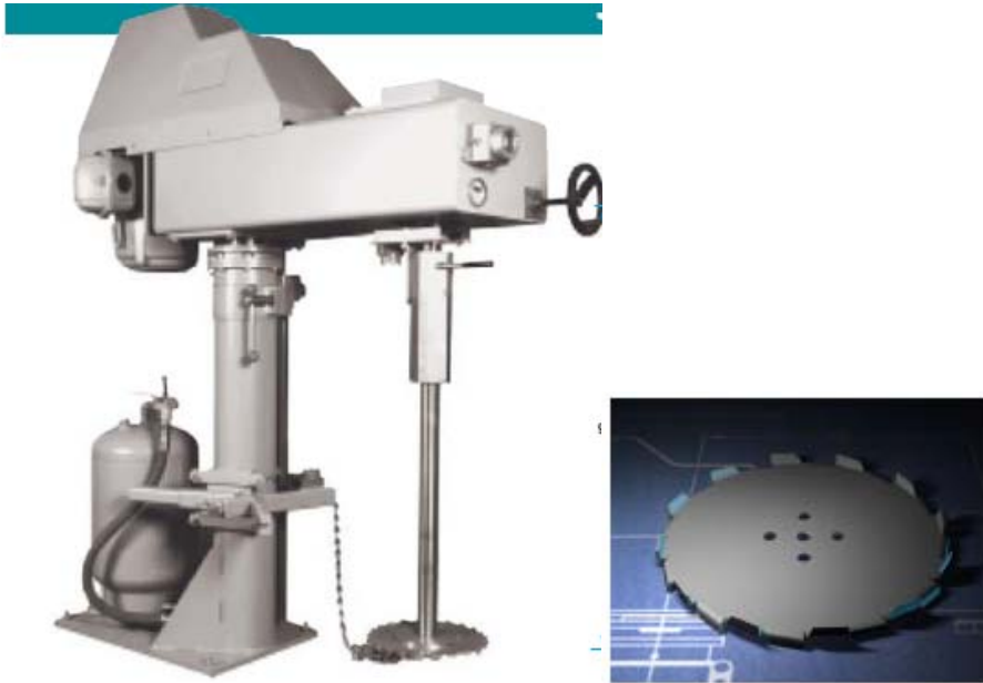
Figure 2. Industrial standard Cowles equipment and "hi-shear" impeller.
