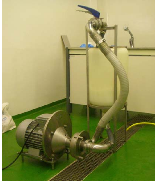
Figure 3. FRISTAM shear pump prototype and ancillary equipment for testing in the MPP.
