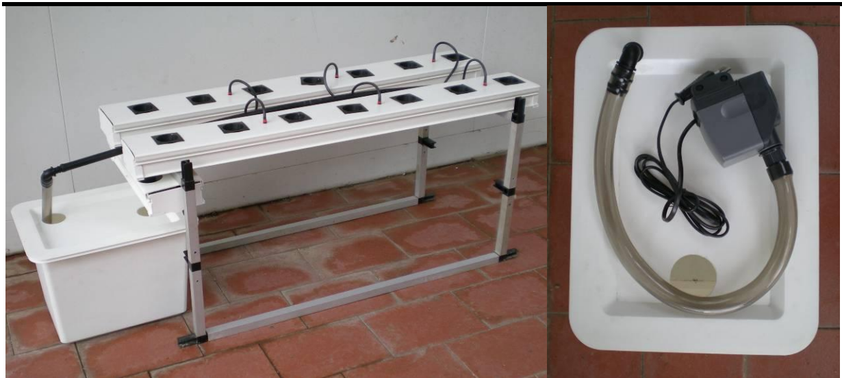
Fig. 55 Views of the double gully, the nutrient solution tank and the submerged pump.
