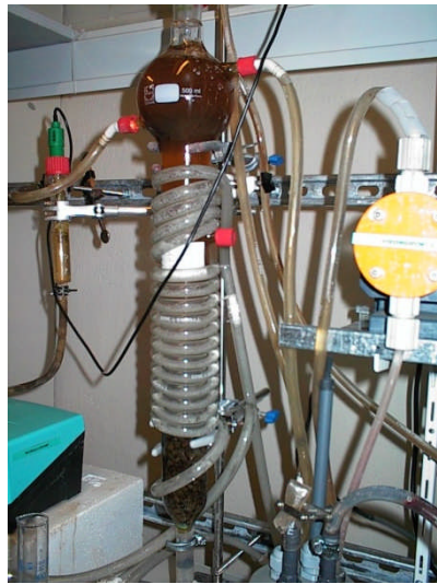
Figure 6. View of the lab-scale methanogenic reactor
