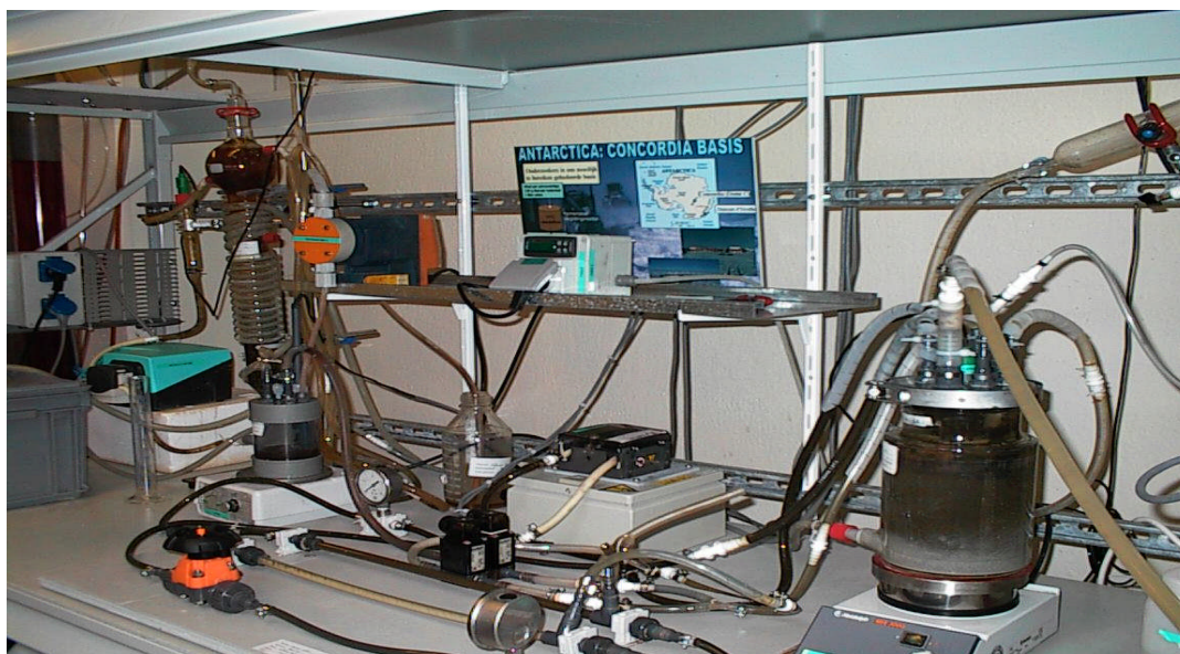
Figure 5. View of the lab-scale set-up. From right to left: Liquefying reactor, Ultrafiltration unit and methanogenic reactor
