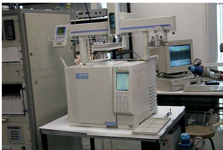
Figure 1 General GC equipment installed at the MELISSA Pilot Plant, UAB.
