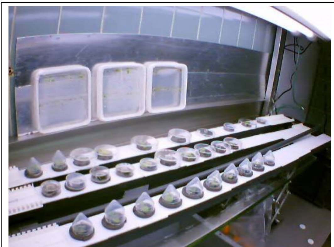
Figure 1: Petri dish germination and NFT propagation setup
