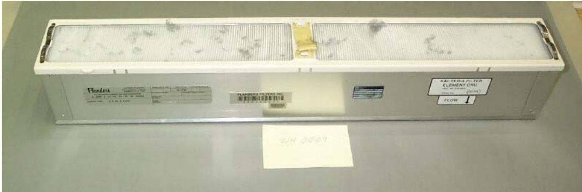
Figure 5-6 Typical Bacteria Filter Element [R18]
