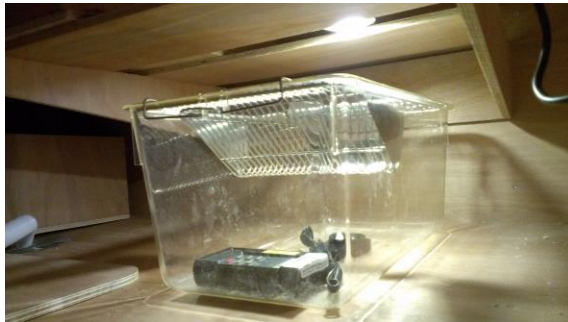
Lux level testing in the wooden mock-up
