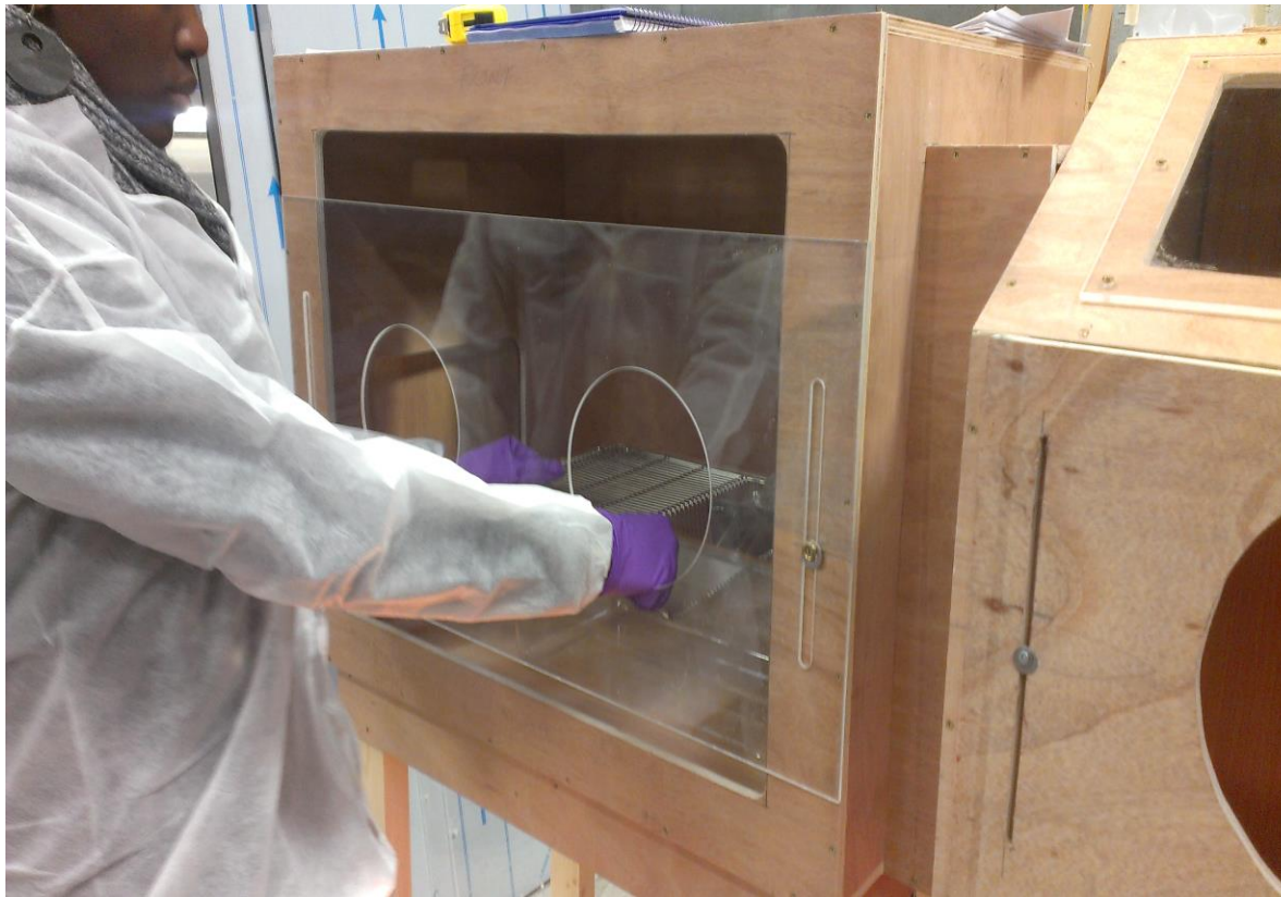
Wooden mock-up used for ergonomic testing and design verification
