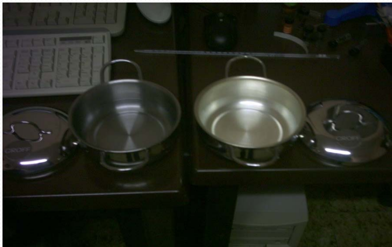
Left pot = AISI 316 Right pot = Silver plated internally 20 micron Ag
