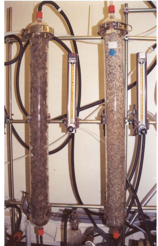
Biofiltration of toluene vapors with Cladophialophora psammophila
