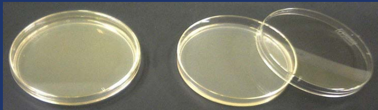
Petri dishes = traditional device for microbial culture Contain agar based culture media (with water)
