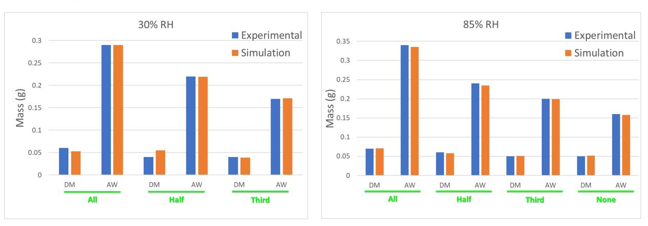
Experimental and simulation results are consistent both in terms of Dry Mass and Accumulate Water
