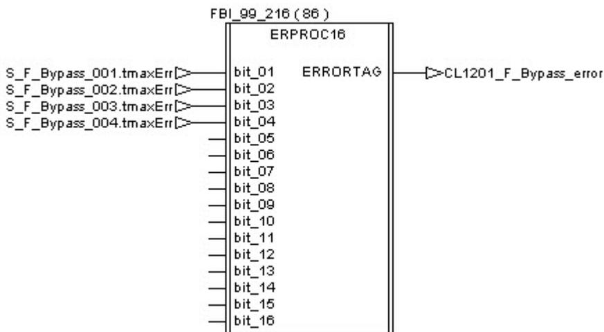
If an error is detected during the execution of the procedure, The tag “CL1201\_F\_Bypas\_error\_Stop” receives a pulse and then the Filtration Unit is stopped thanks to the procedure “F\_Stop”.
