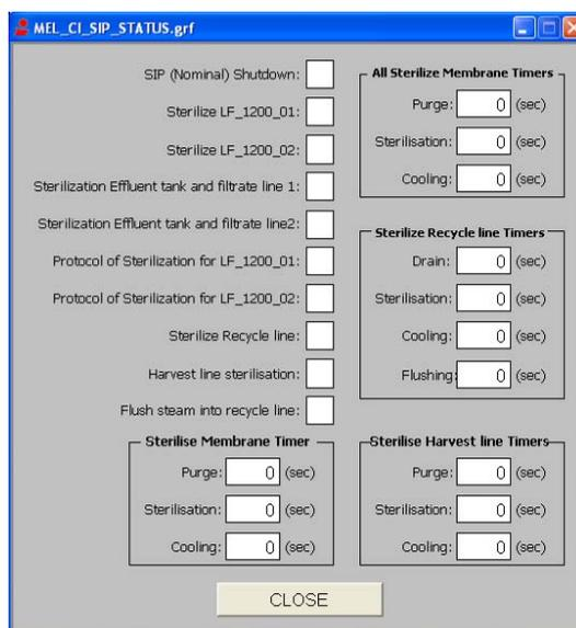
Figure 6-40: Indicators of the SIP procedures
