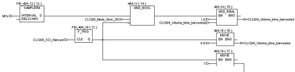
Detects whether flow rate SP was changed during the day because this would cause a faulty calibration.
