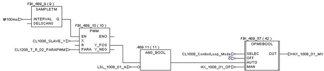
The Slave controller is initialized when the Bioreactor temperature control loop is triggered in Automatic mode.
