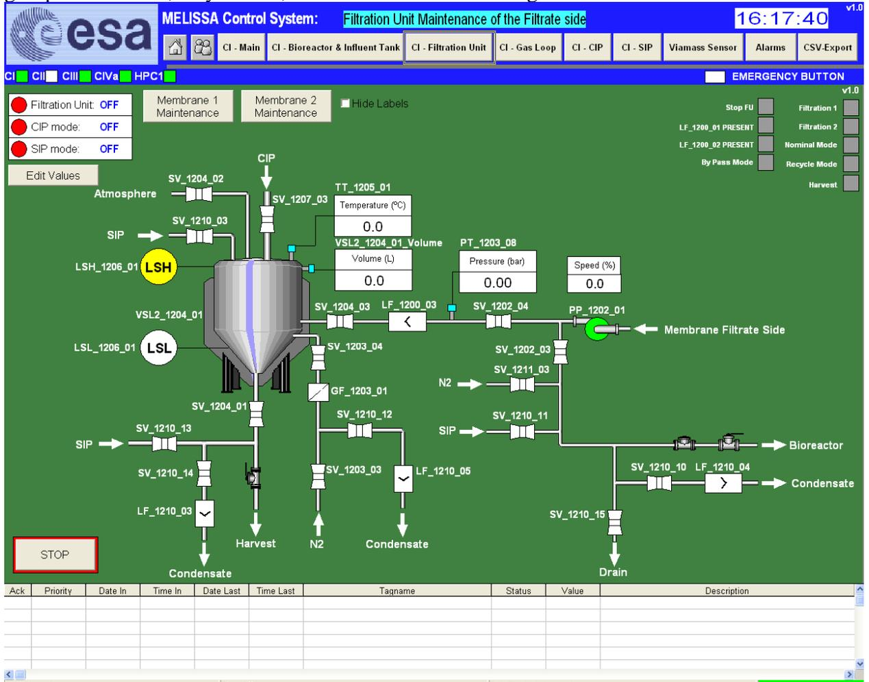
Figure 6-18: Main objects of the Filtration Unit Maintenance screen (Filtrate side)
