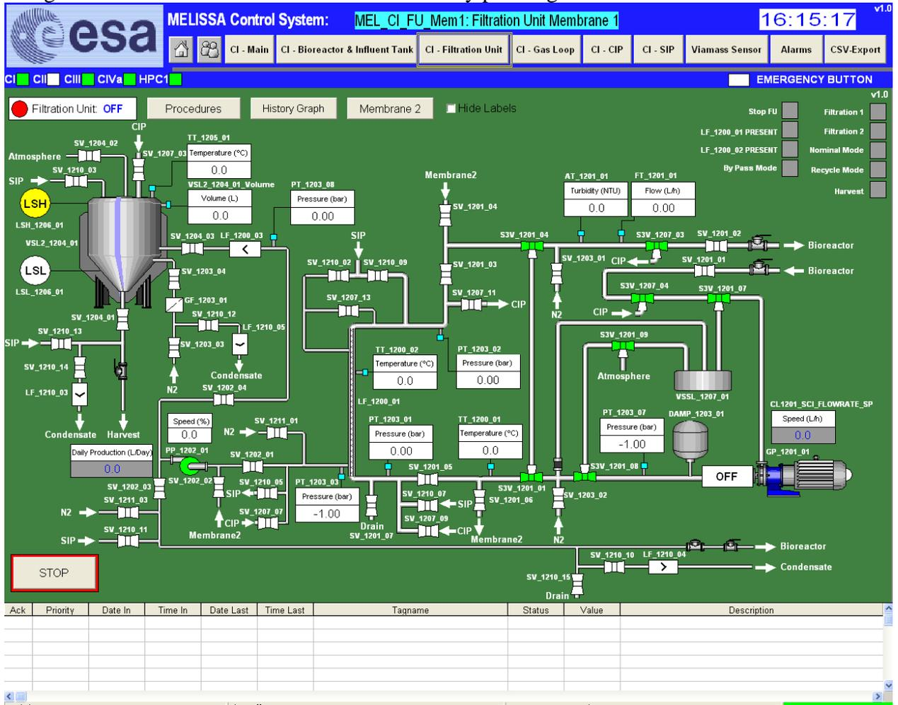
Figure 6-14: Main objects of the Membrane 1 Filtration Unit screen
