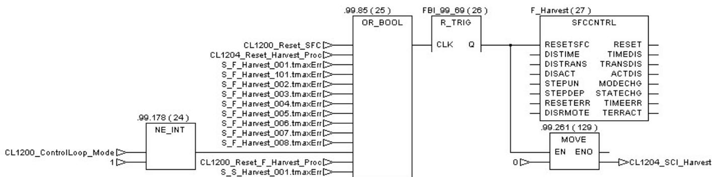
When the procedure starts, a window appears to confirm the harvest choice. The operator can start the harvest or cancel it. The cancel function is done by the following implementation.
