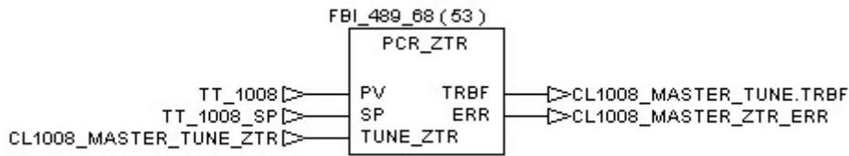
The Master controller is initialized when the Bioreactor temperature control loop is triggered in Automatic mode.
