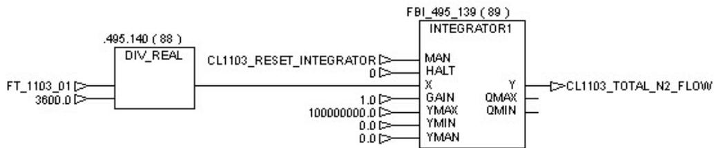
A second calculation is done to know the nitrogen quantity injected during the day. The calculation implemented is a sliding mean value updated each hour.
