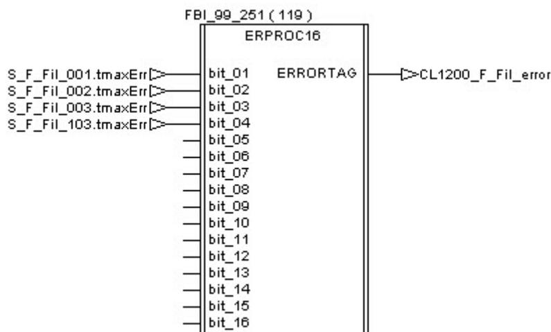
If an error is detected during the execution of the procedure, the tag “CL1201\_F\_Fil\_error\_Stop” receives a pulse then the Filtration Unit is stopped thanks to the procedure “F\_Stop”.
