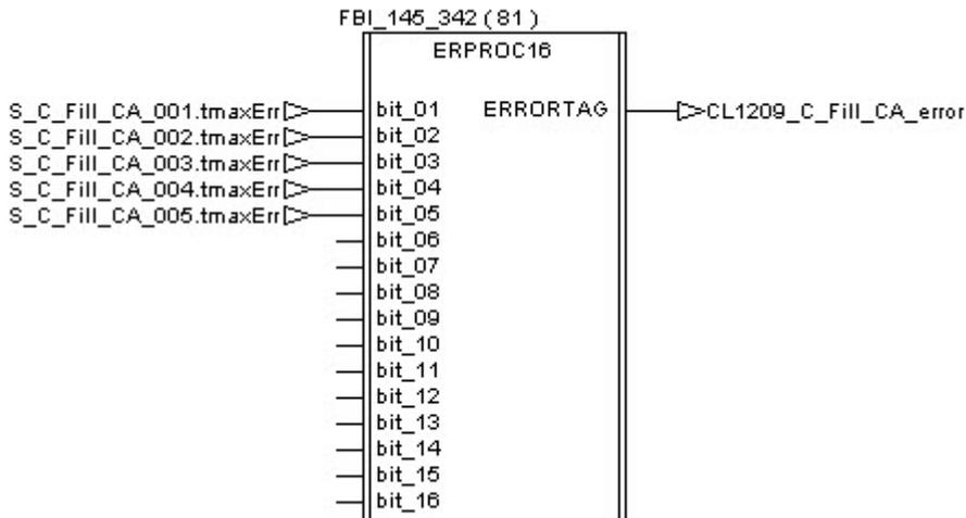
If an error is detected during the execution of the procedure, the tag “CL1207\_C\_FILL\_CA\_error\_Stop” receives a pulse and then the Cleaning Unit is stopped thanks to the procedure “C\_Stop”.
