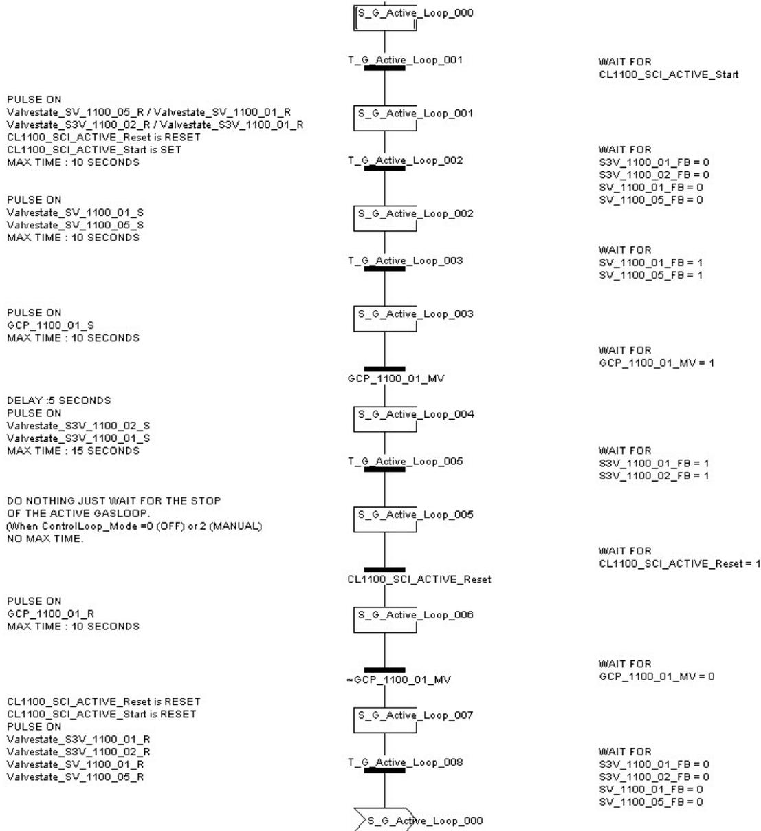
Figure 112: PLC procedure: G\_Active\_Loop
