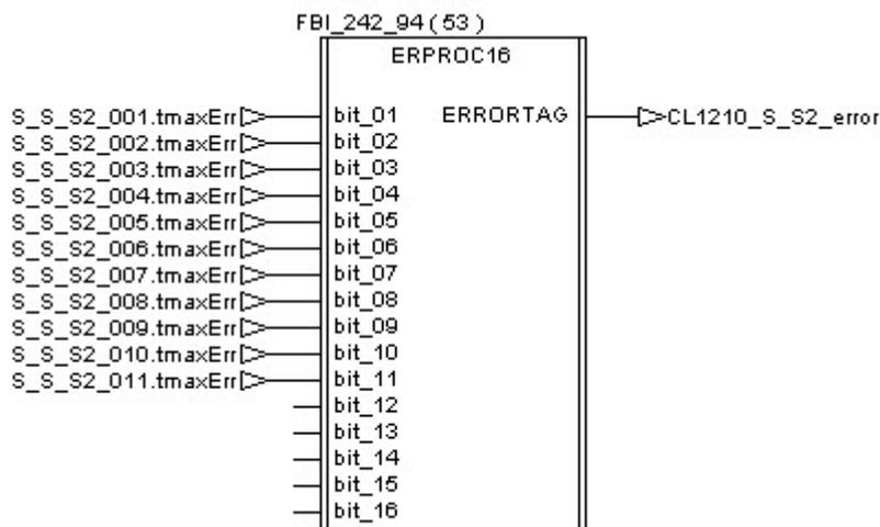
If an error is detected during the execution of the procedure, the tag “CL1210\_S\_S2\_error\_Stop” receives a pulse and then the Sterilization Unit is stopped thanks to the procedure “S\_Stop”.
