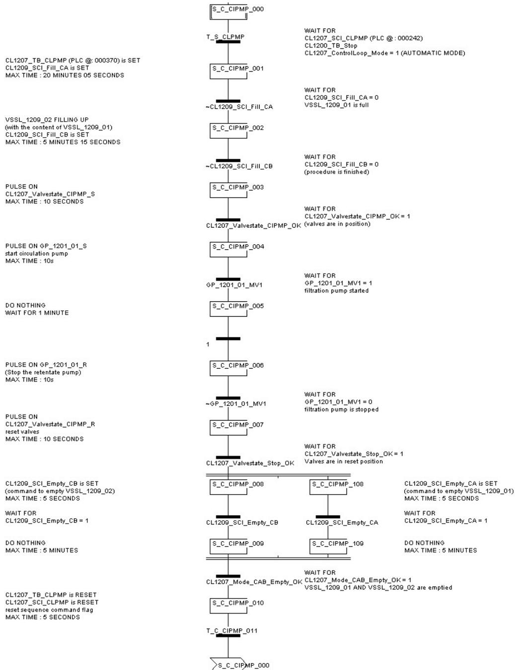
Figure 131: PLC procedure: C\_CLPMP
