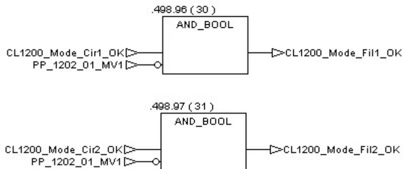
If one of the two modes is set, the following tracing bit is directly set.
