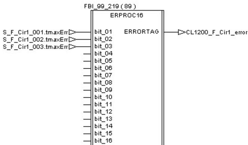
If an error is detected during the execution of the procedure, the tag “CL1200\_F\_Cir1\_error\_Stop” receives a pulse then the Filtration Unit is stopped thanks to the procedure “F\_Stop”.
