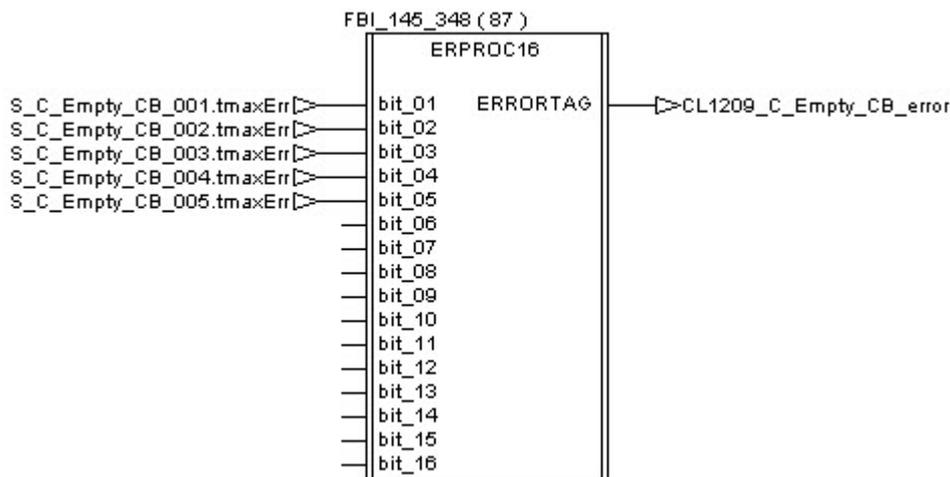
If an error is detected during the execution of the procedure, the tag “CL1207\_C\_EMPTY\_CB\_error\_Stop” receives a pulse and then the Cleaning Unit is stopped thanks to the procedure “C\_Stop”.
