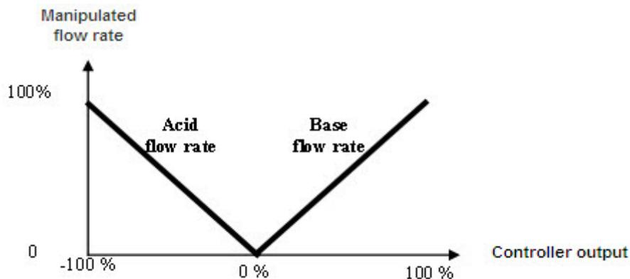
In order to control the pH, the PLC needs to have, at the input of the controller, the process value +/- the dead zone defined by the operator. Depending on the mode pH state (High or low) the dead zone is added (pH high) or subtracted (pH low) to the analyser value.
