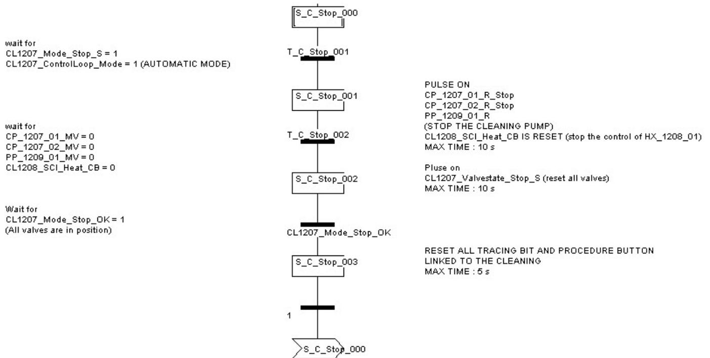
Figure 124: PLC procedure: C\_Stop
