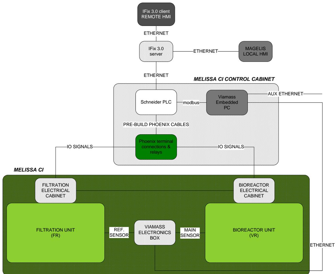
**Figure 2-1: MELISSA CI block diagram with VIAMASS Sensor System.**
