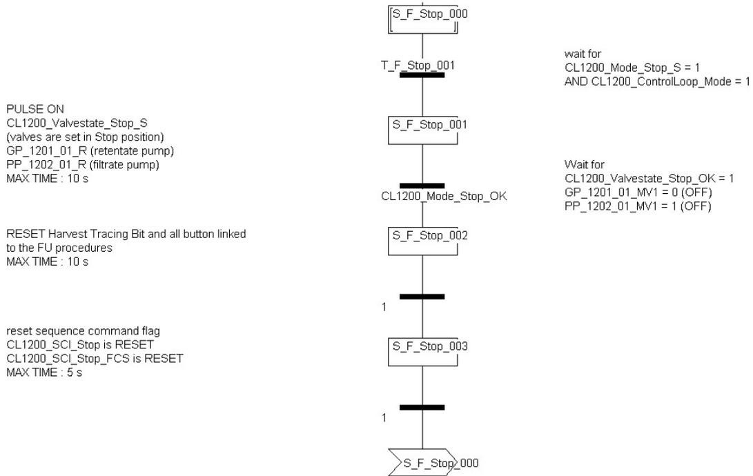
Figure 113: PLC procedure: F\_Stop
