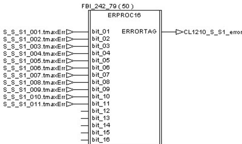
If an error is detected during the execution of the procedure, the tag “CL1210\_S\_S1\_error\_Stop” receives a pulse and then the Sterilization Unit is stopped thanks to the procedure “S\_Stop”.
