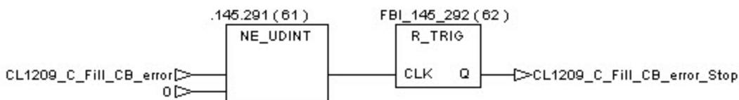
The error number is displayed until the procedure is re-started.
