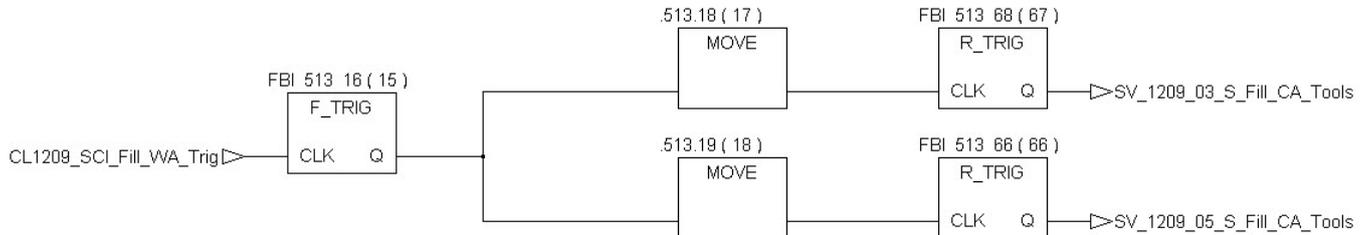
Finally, when VSSL\_1209\_01 is full, the Level switch high LSH\_1209\_01 is reset (inverted logic). The valves SV\_1209\_03 and SV\_1209\_05 are reset by a pulse. The tag “CL1207\_Fill\_WA\_Timeout” (which also reset the valves enounced above) is set if the SV\_1209\_03 (Water entrance) is opened more than 3 minutes.
