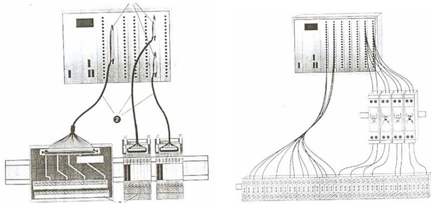
**Figure 10 PHOENIX VARIOFACE PLUGGABLE SYSTEM vs TRADITIONAL WIRING SYSTEM**
