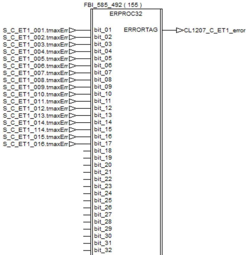
If an error is detected during the execution of the procedure, the tag “CL1207\_C\_ET1\_error\_Stop” receives a pulse and then the Cleaning Unit is stopped thanks to the procedure “C\_Stop”.
