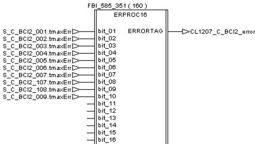
If an error is detected during the execution of the procedure, the tag “CL1207\_C\_BCI2\_error\_Stop” receives a pulse and then the Cleaning Unit is stopped thanks to the procedure “C\_Stop”.
