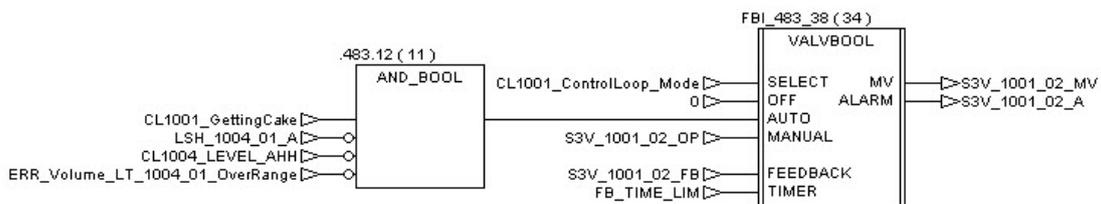
**During the get cake function, the Valve S3V\_1001\_01, which permits to inject influent content inside the bioreactor, is forced in default position. It protects the bioreactor from direct injection of fresh wastes.**
