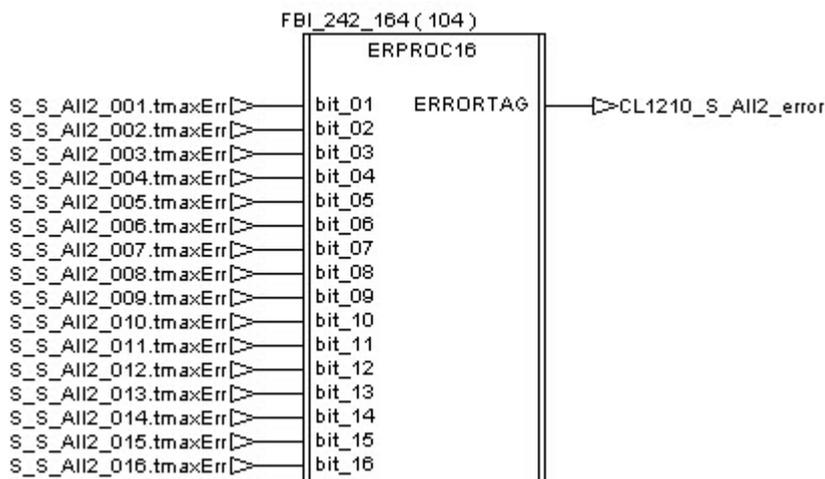
If an error is detected during the execution of the procedure, the tag “CL1210\_S\_ALL2\_error\_Stop” receives a pulse and then the Sterilization Unit is stopped thanks to the procedure “S\_Stop”.
