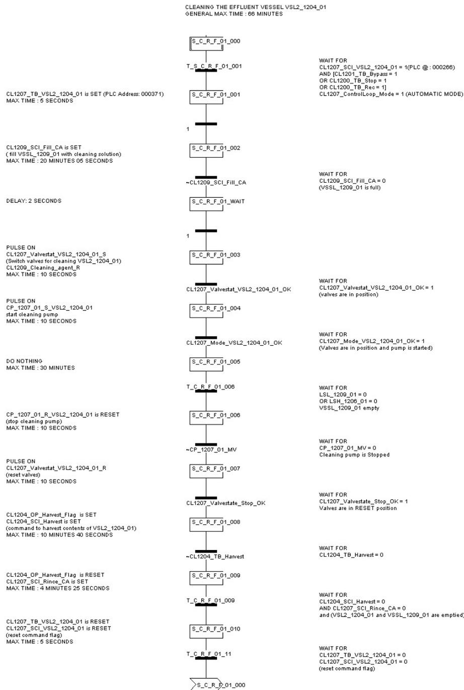
Figure 132: PLC procedure: C\_R\_F\_01
