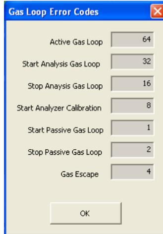
Figure 6-13: Error Codes of the Gas Loop Procedures
