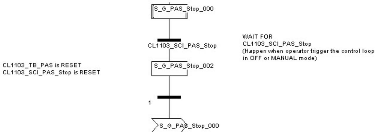
Figure 106 : PLC procedure G\_PAS\_Stop
