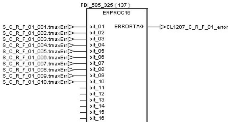
If an error is detected during the execution of the procedure, the tag “CL1207\_C\_R\_F01\_error\_Stop” receives a pulse and then the Cleaning Unit is stopped thanks to the procedure “C\_Stop”.
