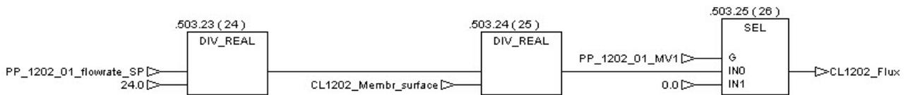
Flux = Filtrate flow rate [L/h] / membrane surface [m<sup>2</sup>]
