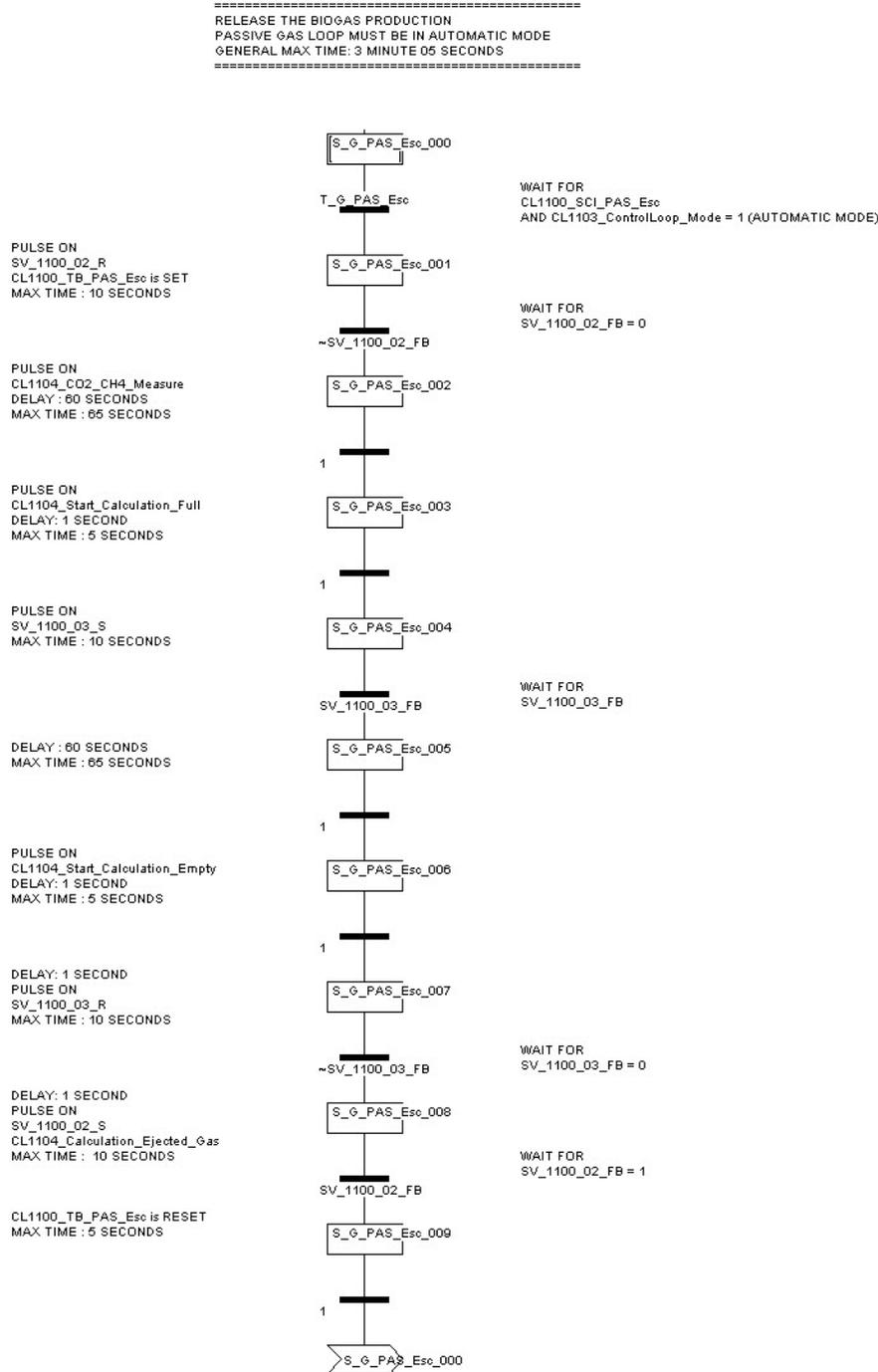
Figure 108: PLC procedure: G\_PAS\_Esc
