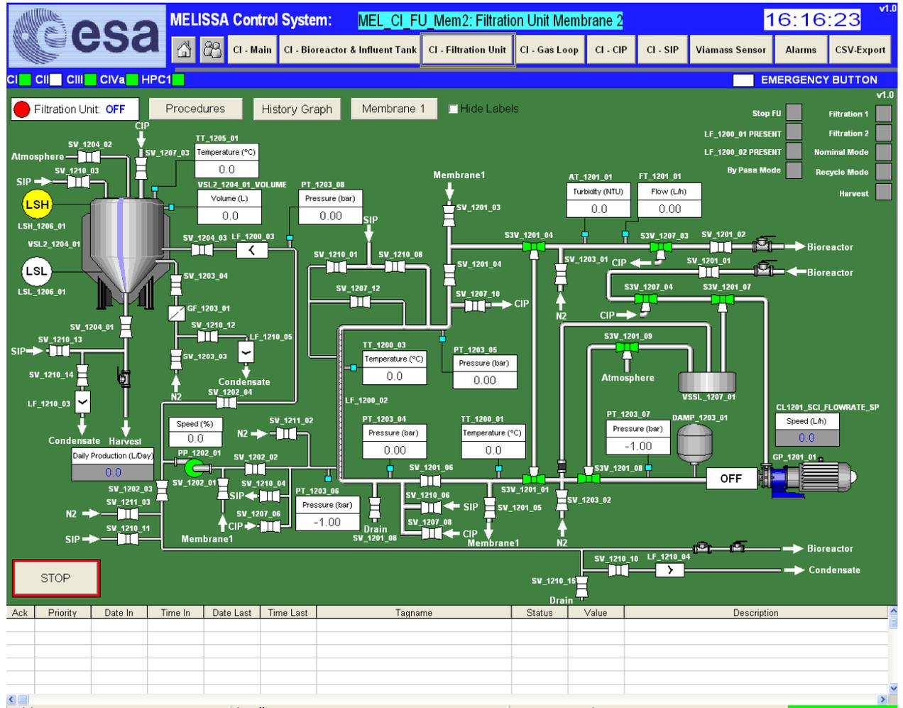
Figure 6-17: Main objects in Membrane 2 Filtration Unit screen
