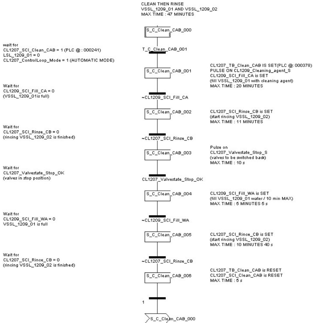
Figure 140: PLC procedure: C\_Clean\_CAB
