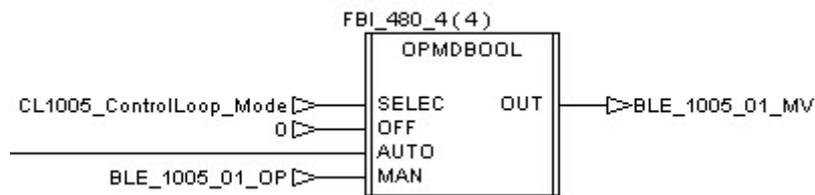
Internally, three selector blocks manage the input which will control the output.
