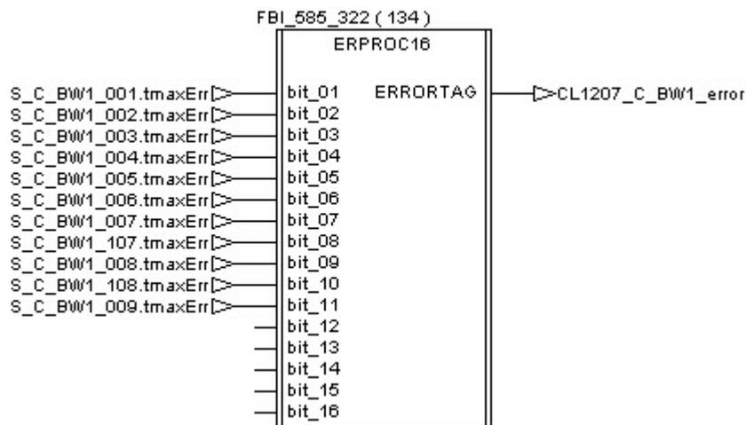
If an error is detected during the execution of the procedure, the tag “CL1207\_C\_BW1\_error\_Stop” receives a pulse and then the Cleaning Unit is stopped thanks to the procedure “C\_Stop”.
