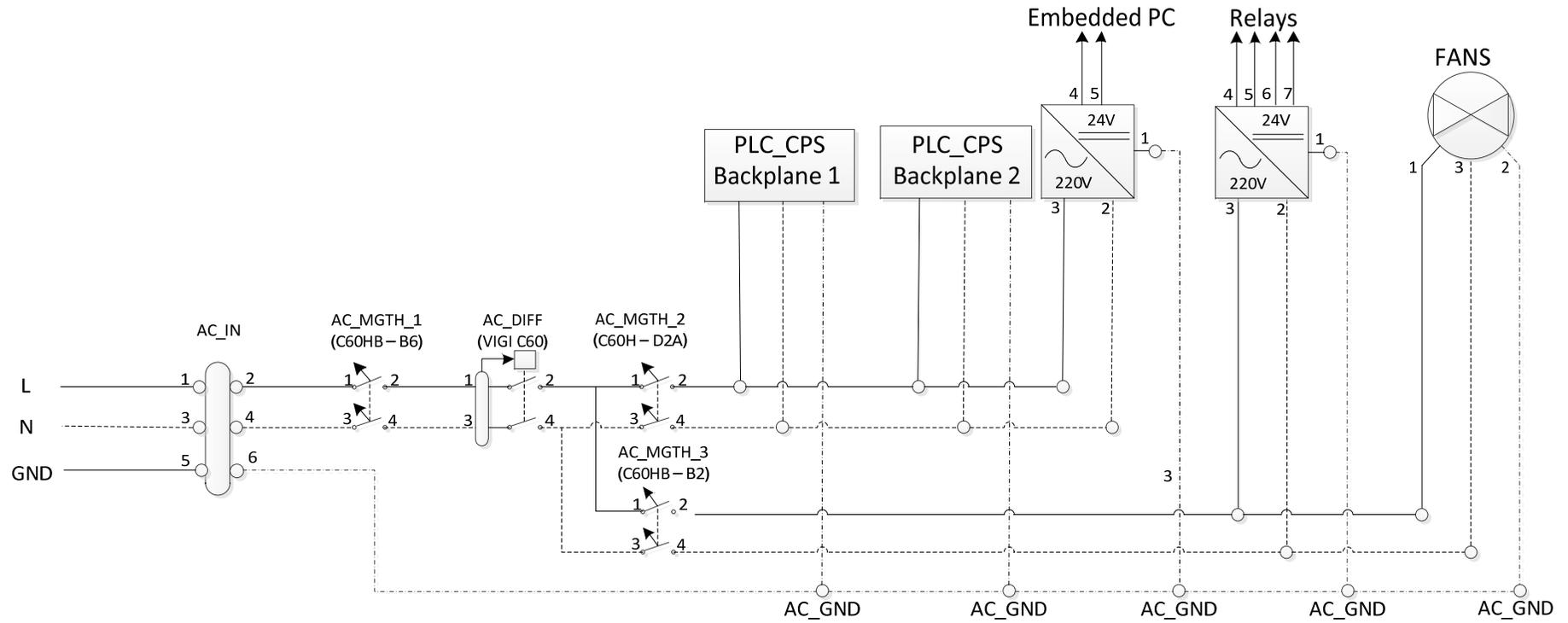
**Figure9 CI Control Cabinet Power Distribution Schematic**
