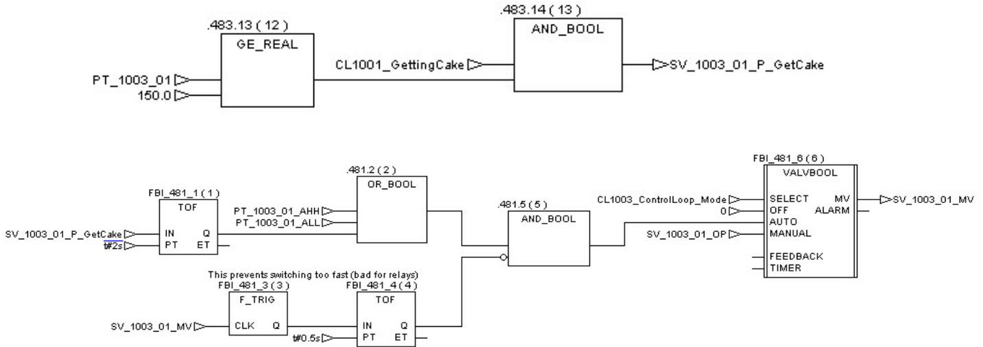
As the valve has no Feedback, the block 'VALVBOOL' (Described in annex) is not configured to trigger any valve alarm. The alarm is set after 5 seconds if the Influent pressure is still greater than 10 mbar with the valve opened.
