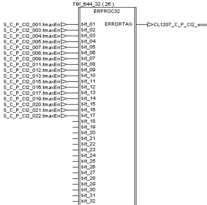
If an error is detected during the execution of the procedure, the tag “CL1207\_C\_P\_Ci2\_error\_Stop” receives a pulse and then the Cleaning Unit is stopped thanks to the procedure “C\_Stop”.
