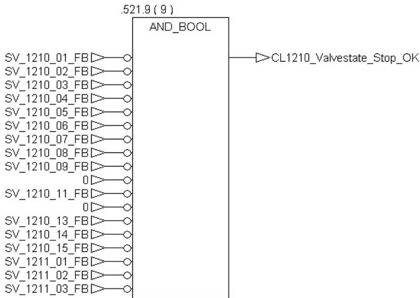
When all the valves are in default position, the tag “CL1210\_Mode\_Stop\_OK” is set.
