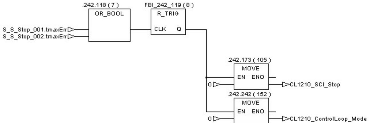
In Parallel, the procedure named “CL1210\_RESET\_PROC” is started. This procedure, detailed further on, triggers a general reset (SIP procedures and equipments) to ensure the default status of all the Sterilization functions when automatic mode is re-started.
