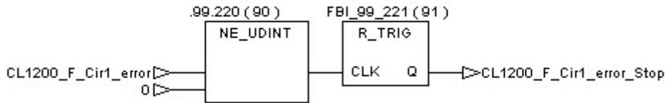
The error number is displayed until the procedure is re-started.
