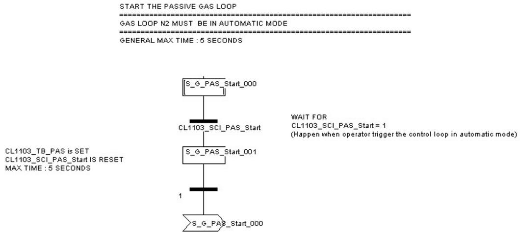
Figure 107: PLC procedure: G\_PAS\_Start
