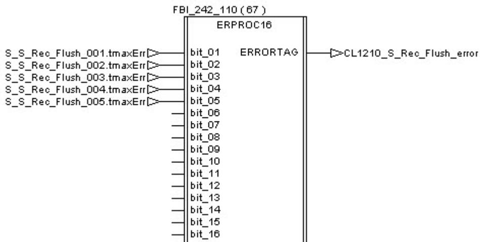
If an error is detected during the execution of the procedure, the tag “CL1210\_S\_REC\_Flush\_error\_Stop” receives a pulse and then the Sterilization Unit is stopped thanks to the procedure “S\_Stop”.
