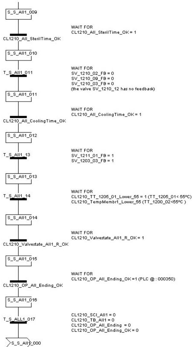
Figure 149: PLC procedure: S\_All1
