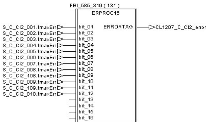
If an error is detected during the execution of the procedure, the tag “CL1207\_C\_Ci2\_error\_Stop” receives a pulse and then the Cleaning Unit is stopped thanks to the procedure “C\_Stop”.
