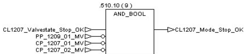
Finally, when “CL1207\_Mode\_Stop\_OK” and all procedures are reset, the Tracing Bit “CL1207\_TB\_Stop” is set.
