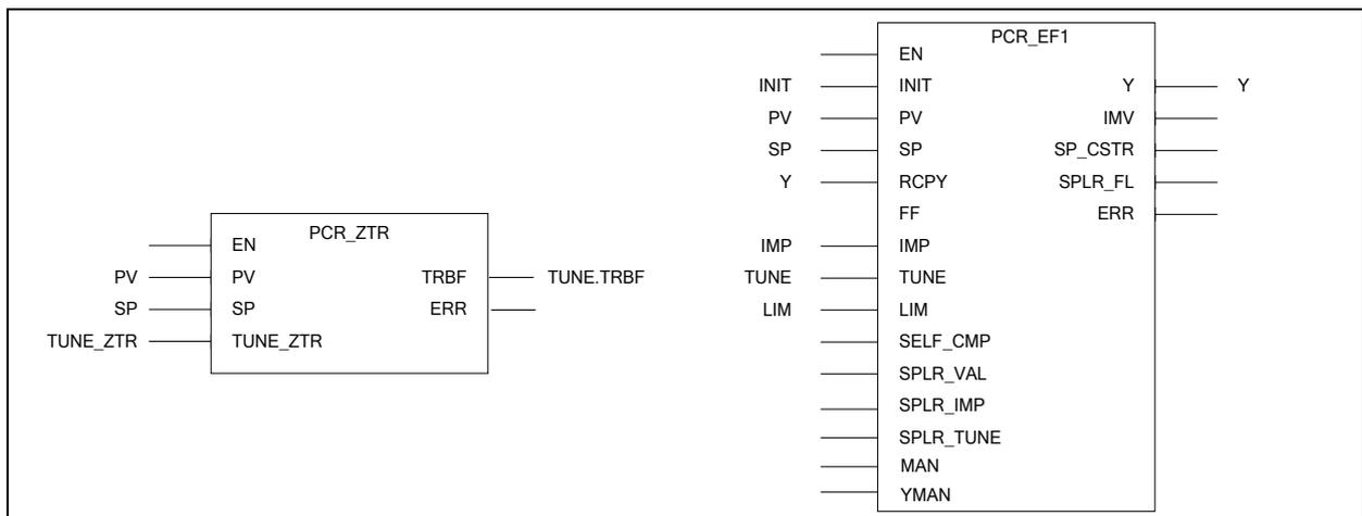
Figure 164: Use of zone control with a PCR\_EF1 block
