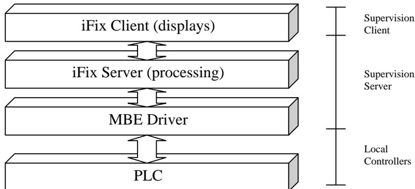
The MBE driver runs in the Supervision Server. This application uses Modbus over TCP/IP to communicate with the PLC. The configuration of the driver is edited with the MBE Power Tool, this application can be accessed directly from the iFix Database Manager. The resulting file defines the configuration of the blocks of information transferred from/to the PLC.
