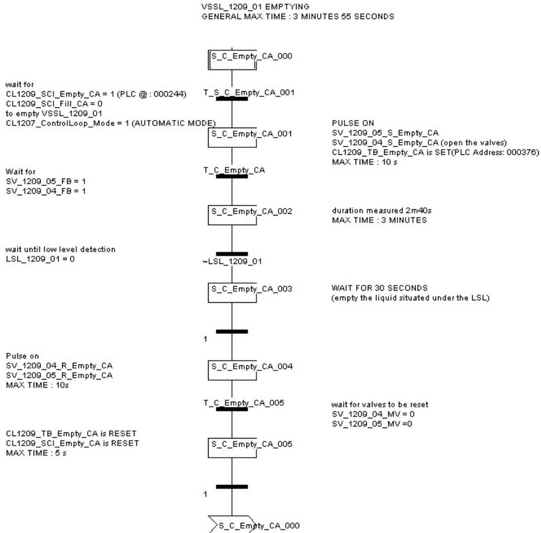
Figure 138: PLC procedure: C\_Empty\_CA
