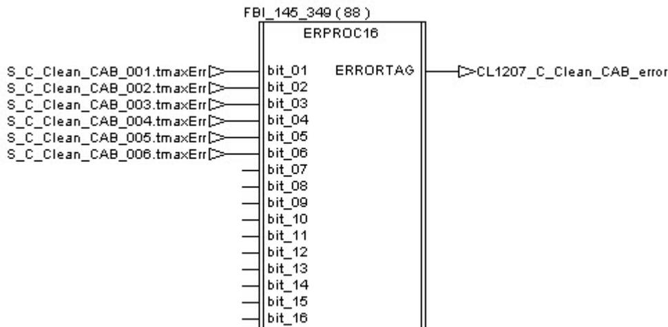
If an error is detected during the execution of the procedure, the tag “CL1207\_C\_CLEAN\_CAB\_error\_Stop” receives a pulse and then the Cleaning Unit is stopped thanks to the procedure “C\_Stop”.
