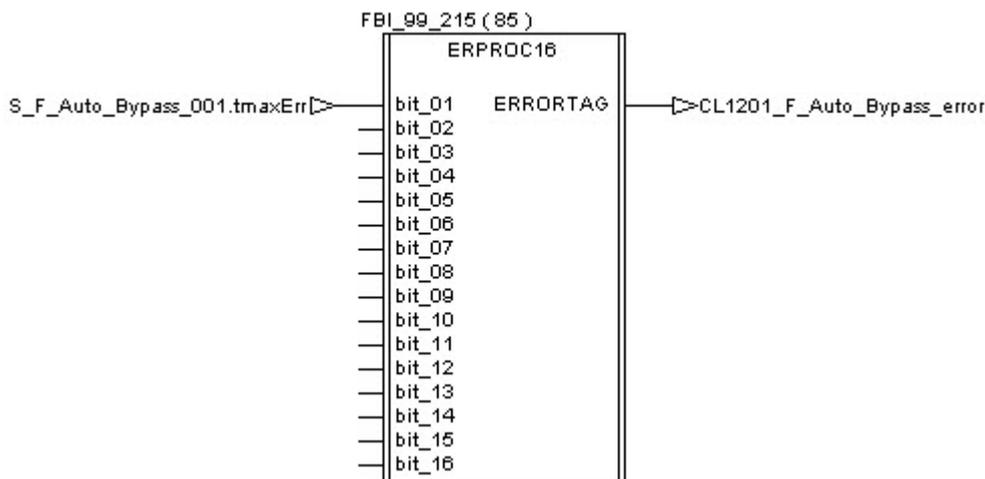
If an error is detected during the execution of the procedure, the tag “CL1201\_F\_AUTO\_Bypas\_error\_Stop” receives a pulse and then the Filtration Unit is stopped thanks to the procedure “F\_Stop”.
