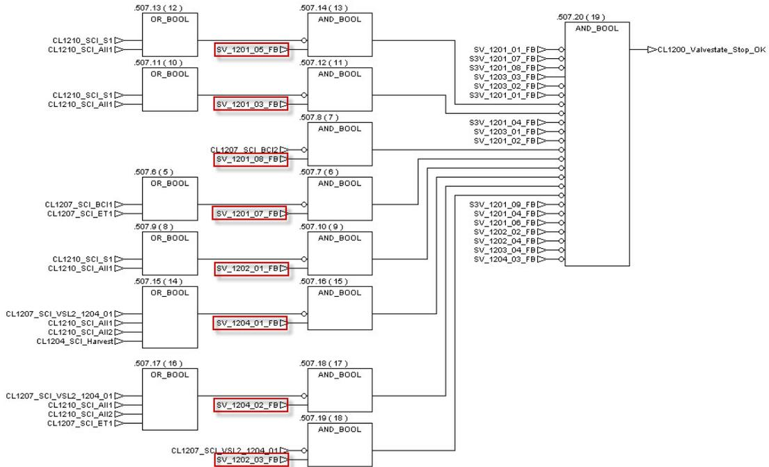
Because some filtration valves are also managed by Cleaning or sterilization procedure, the variable “CL1200\_Valvestate\_Stop\_OK” can be set even if some valves are not in default position. These valves are surrounded by a red rectangle.
