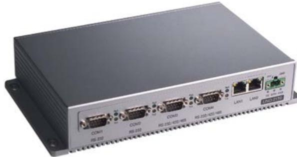
Embedded pc is the interface between biomass sensor and PLC. The current version takes data from biomass sensor box (bioimpedance value) and sends it to the plc through serial modbus. In future version, it will estimate the biomass present in the bioreactor. For further information see NTE-VSS-HB-017 and NTE-VSS-HB-018 documents.
