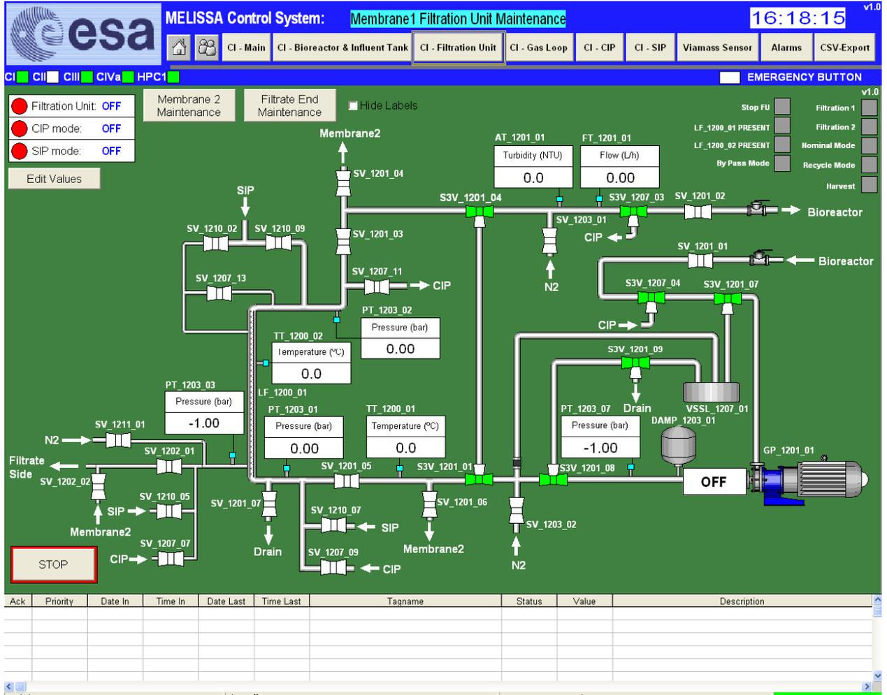
Figure 6-21: Main objects of the Filtration Unit Maintenance screen (Membrane 1 side)
