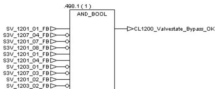
Once done, the pump is started by the procedure. If no failure happens, the tag CL1200\_Mode\_Bypass\_OK is set at the same time than the Tracing bit.
