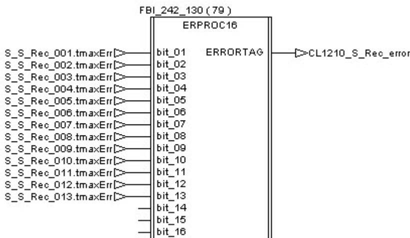
If an error is detected during the execution of the procedure, the tag “CL1210\_S\_REC\_error\_Stop” receives a pulse and then the Sterilization Unit is stopped thanks to the procedure “S\_Stop”.
