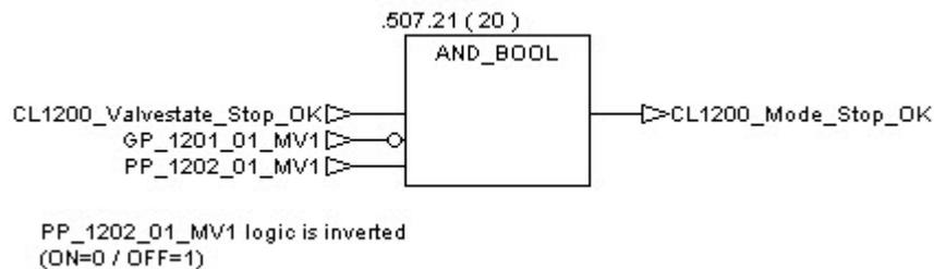
Finally, when “CL1200\_Mode\_Stop\_OK” and all procedures are reset, the Tracing Bit “CL1200\_TB\_Stop” is set.
