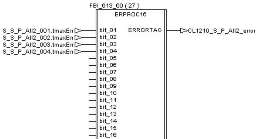
If an error is detected during the execution of the procedure, the tag “CL1210\_S\_P\_ALL2\_error\_Stop” receives a pulse and then the Sterilization Unit is stopped thanks to the procedure “S\_Stop”.
