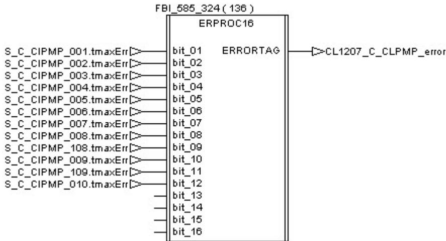
If an error is detected during the execution of the procedure, the tag “CL1207\_C\_CLPMP\_error\_Stop” receives a pulse and then the Cleaning Unit is stopped thanks to the procedure “C\_Stop”.
