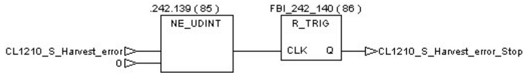
The error number is displayed until the procedure is re-started.
