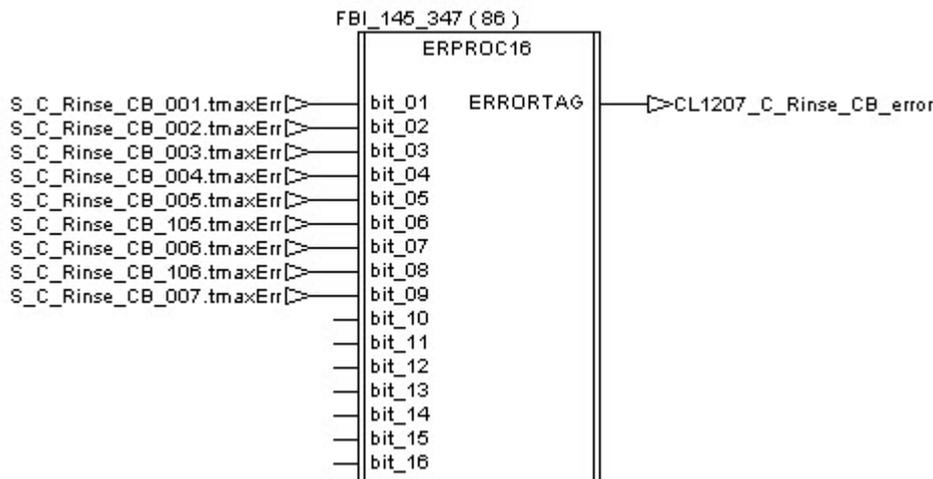
If an error is detected during the execution of the procedure, the tag “CL1207\_C\_RINSE\_CB\_error\_Stop” receives a pulse and then the Cleaning Unit is stopped thanks to the procedure “C\_Stop”.
