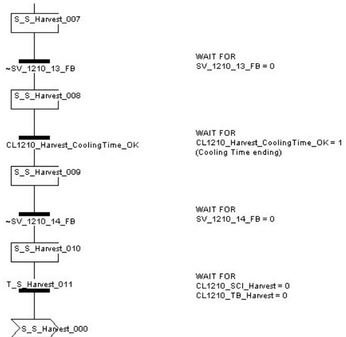
Figure 152: PLC procedure: S\_Harvest
