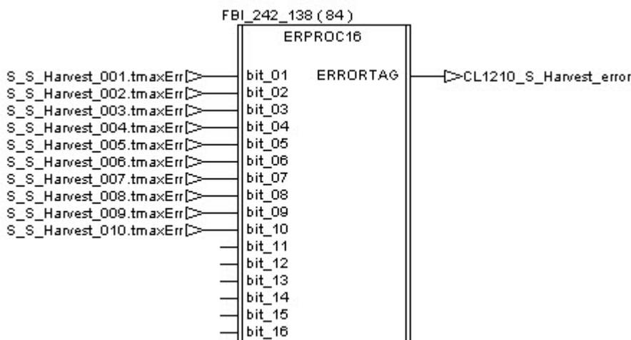
If an error is detected during the execution of the procedure, the tag “CL1210\_S\_Harvest\_error\_Stop” receives a pulse and then the Sterilization Unit is stopped thanks to the procedure “S\_Stop”.
