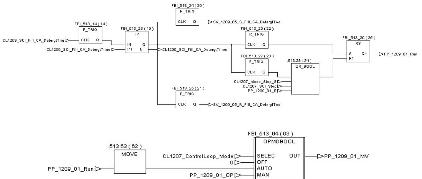
At the end of the time the pump is stopped, then water is added thanks to the procedure C\_Fill\_WA making a pulse on the tag “CL1209\_SCI\_Fill\_WA\_Trigger” (SV\_1209\_03 and SV\_1209\_05 opening).
