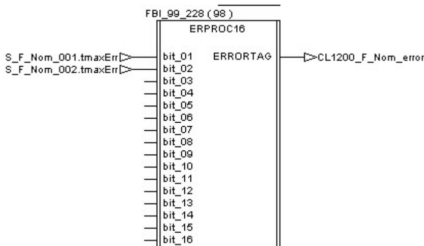
If an error is detected during the execution of the procedure, the tag “CL1200\_F\_Nom\_error\_Stop” receives a pulse and then the Filtration Unit is stopped thanks to the procedure “F\_Stop”.
