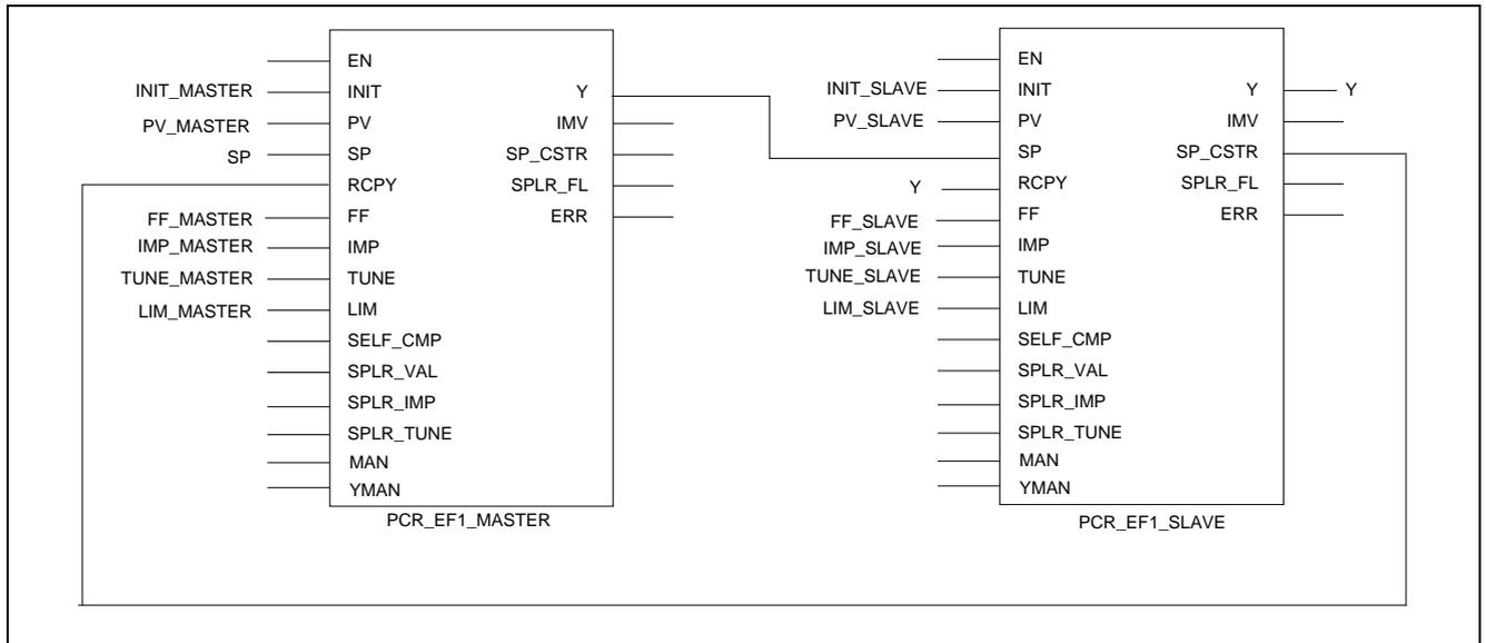
**Figure 159: Example of cascade configuration, using PCR\_EF1 blocks**
