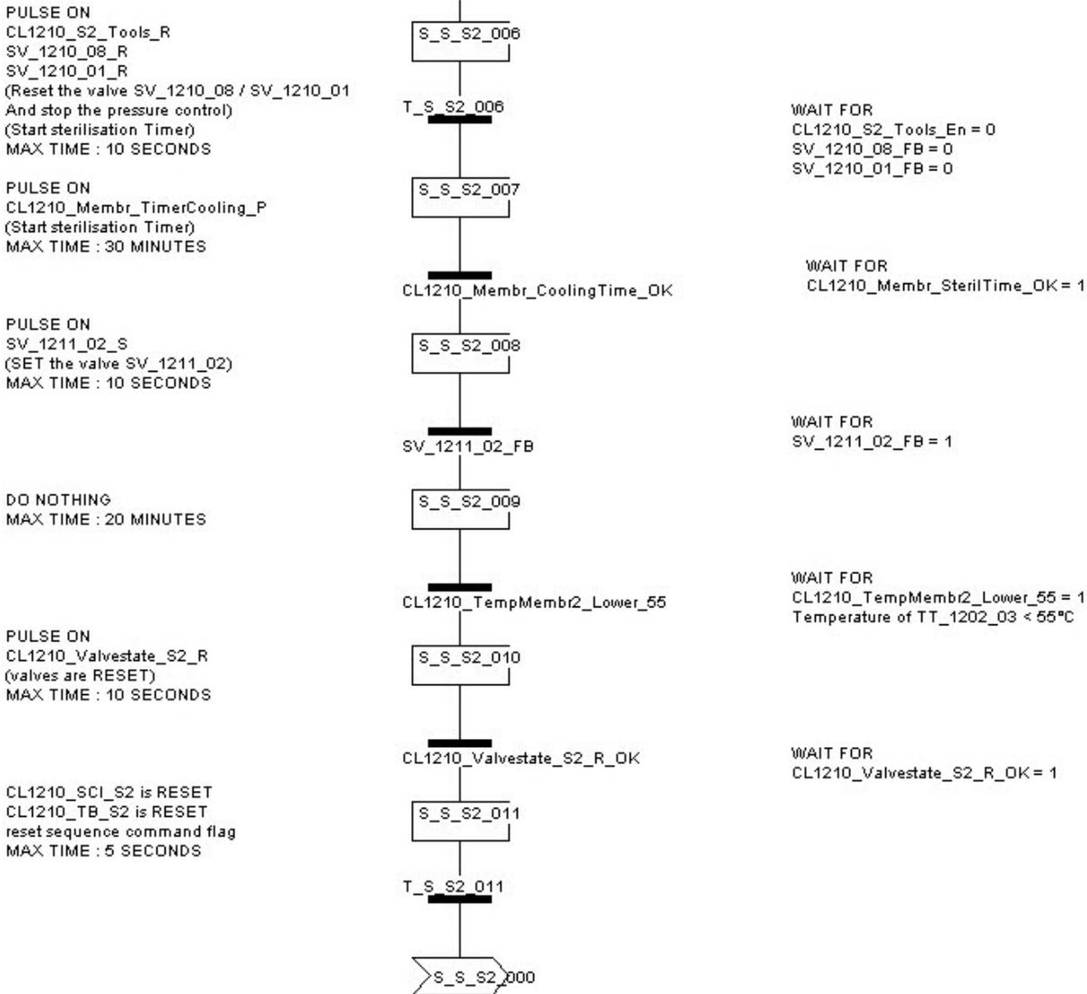
Figure 148: PLC procedure: S\_S2
