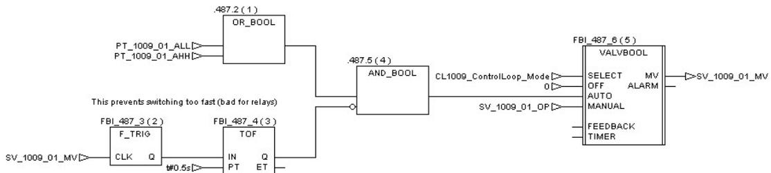
As the valve has no FB, we have changed the way to trigger the alarm. If the valve is open during 5 seconds and the pressure is upper than 10 mBar, the alarm is SET. This alarm happens only if the pressure probe is not in error.
