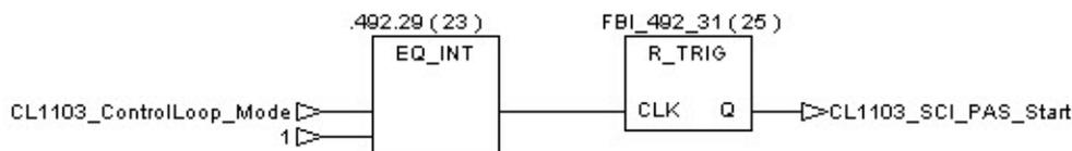
When the operator triggers the Control Loop to OFF or Manual Mode, the procedure “G\_PAS\_Stop” (Detailed in the Chapter 4 “User Manual Procedure”) is called. The tracing Bit of the Passive Gas Loop is RESET.
