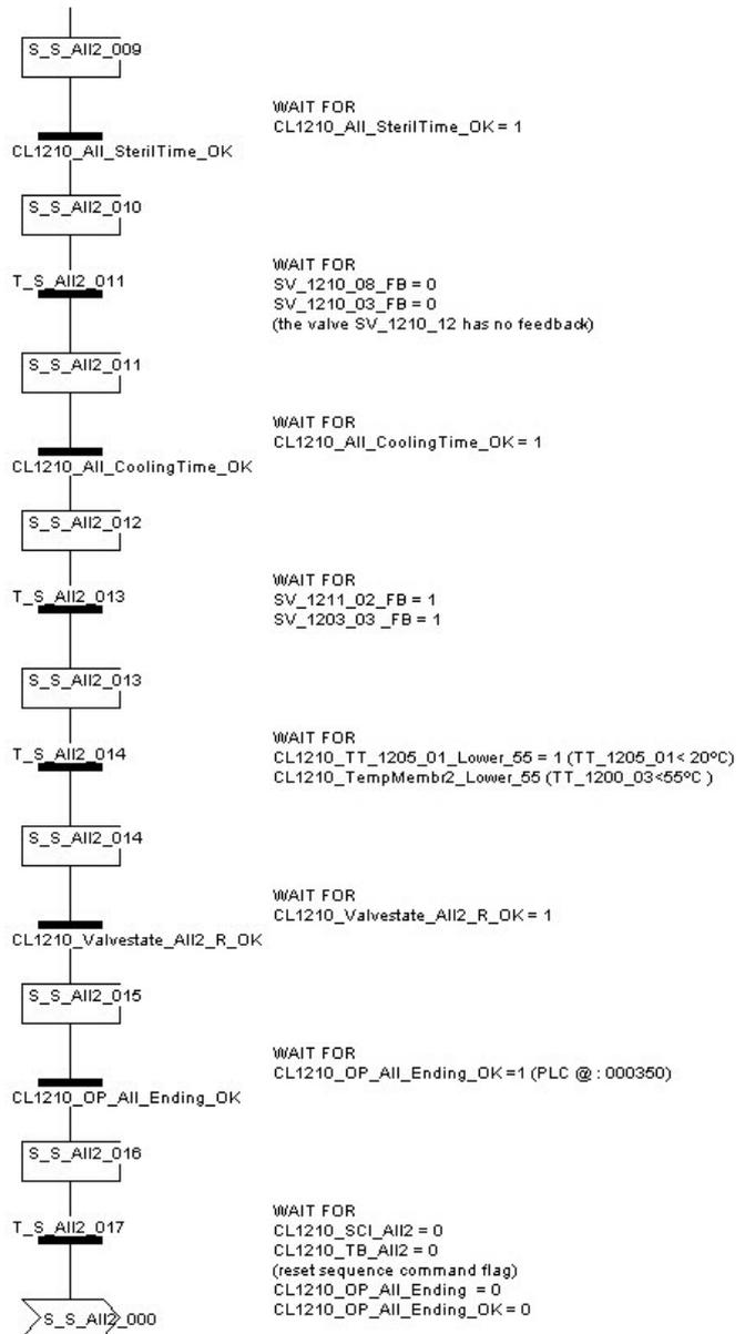
Figure 150: PLC procedure: S\_AII2
