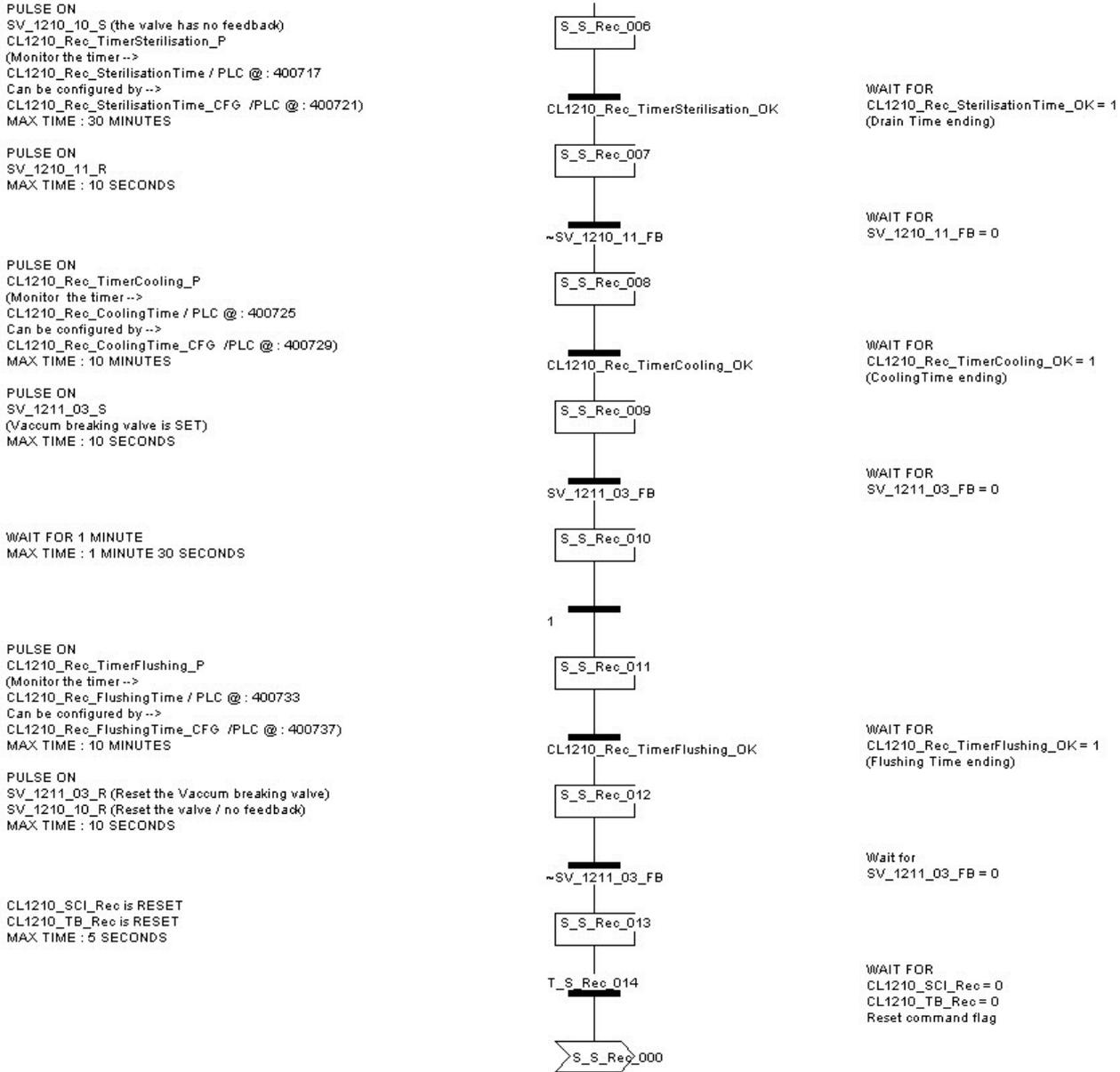
Figure 151: PLC procedure: S\_Rec
