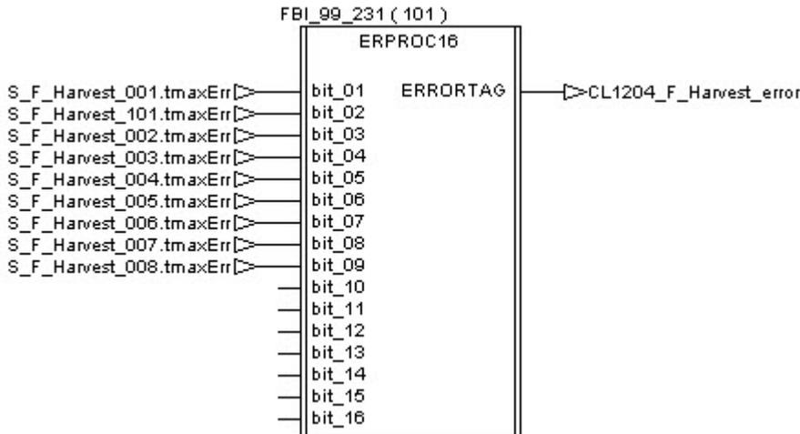
If an error is detected during the execution of the procedure, the tag “CL1204\_F\_Harvest\_error\_Stop” receives a pulse and then the Filtration Unit is stopped thanks to the procedure “F\_Stop”.
