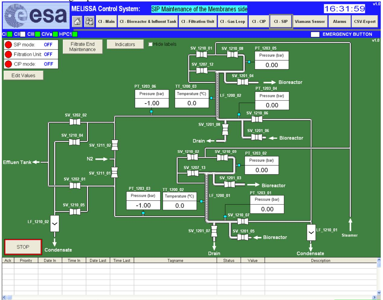
Figure 6-43: Main objects of the SIP Maintenance (Membranes side)
