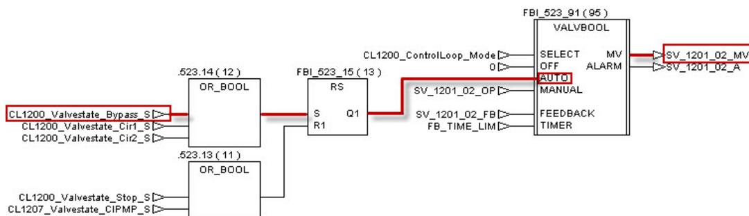
Depending on the procedure step needs, the “\_S”, situated at the end of the tag name, will set the valves in good position (either open or close), as well for the “\_R” which will reset the valves in the default position.
