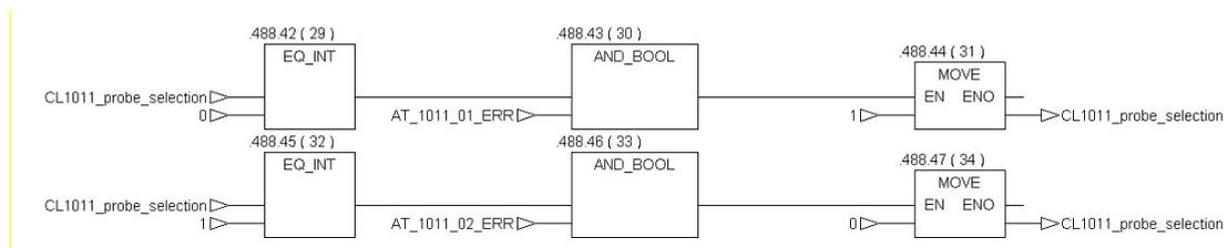
If both probes are in failure, the pH mode is triggered to OFF.
