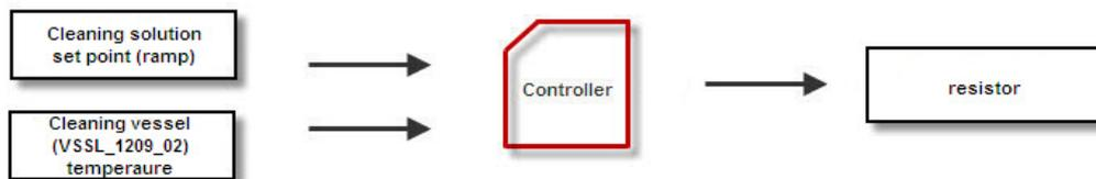
The control is provided by a PI controller. The cleaning solution is warmed until the defined temperature set point thanks to the resistor HX\_1208\_01. A ramp function ensures that no high temperature shock happens to the membrane (30°C delta-T and 10°C/min). This resistor warms the water circulating in the jacket of the cleaning buffer vessel VSSL\_1209\_02.
