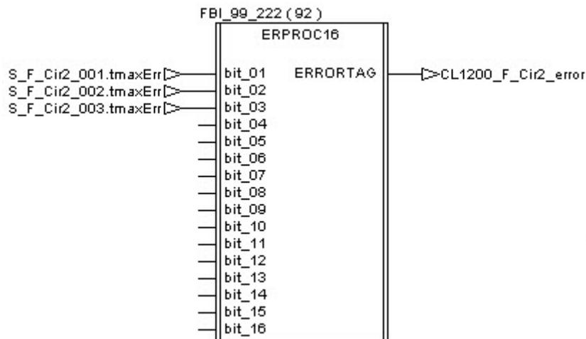
If an error is detected during the execution of the procedure, the tag “CL1200\_F\_Cir2\_error\_Stop” receives a pulse then the Filtration Unit is stopped thanks to the procedure “F\_Stop”.
