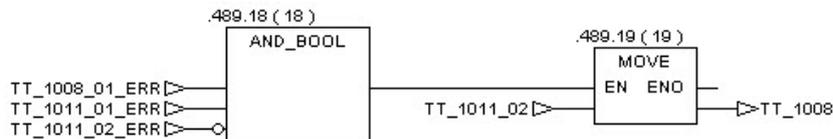
When no bioreactor temperature probes can be used for control, or if the bioreactor blender is in alarm, the PLC send to the slave controller (the one which manages the warm water bath temperature) the set point entered by the operator with 2 °C more. This set point is not displayed on HMI.
