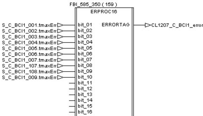
If an error is detected during the execution of the procedure, the tag “CL1207\_C\_BC11\_error\_Stop” receives a pulse and then the Cleaning Unit is stopped thanks to the procedure “C\_Stop”.
