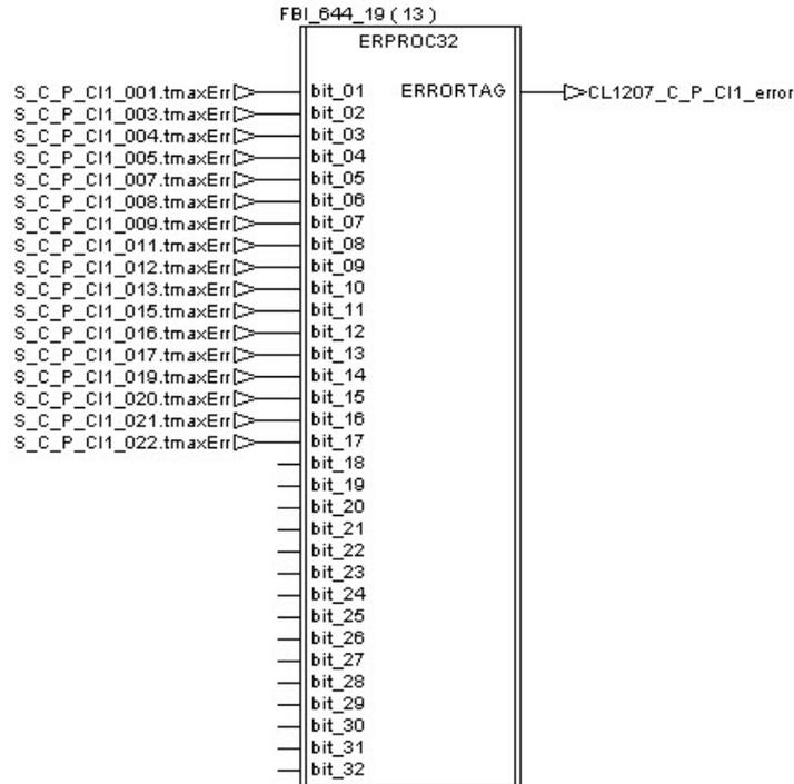
If an error is detected during the execution of the procedure, the tag “CL1207\_C\_P\_CI1\_error\_Stop” receives a pulse and then the Cleaning Unit is stopped thanks to the procedure “C\_Stop”.
