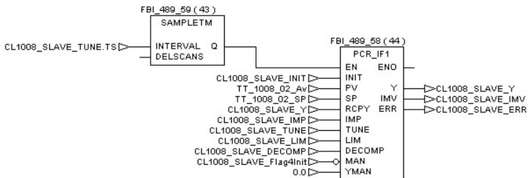
The output of the slave controller is converted into a time binary signal by a PWM block (see annex) to command the resistor.
