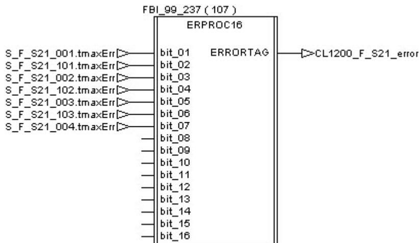
If an error is detected during the execution of the procedure, the tag “CL1200\_F\_S12\_error\_Stop” receives a pulse and then the Filtration Unit is stopped thanks to the procedure “F\_Stop”.
