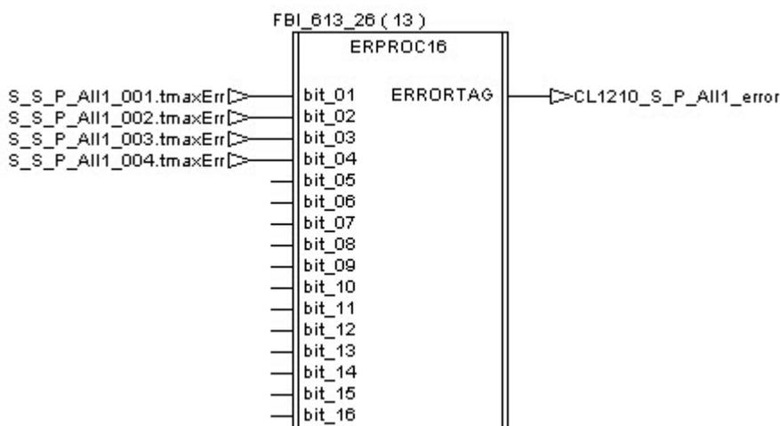
If an error is detected during the execution of the procedure, the tag “CL1210\_S\_P\_ALL1\_error\_Stop” receives a pulse and then the Sterilization Unit is stopped thanks to the procedure “S\_Stop”.
