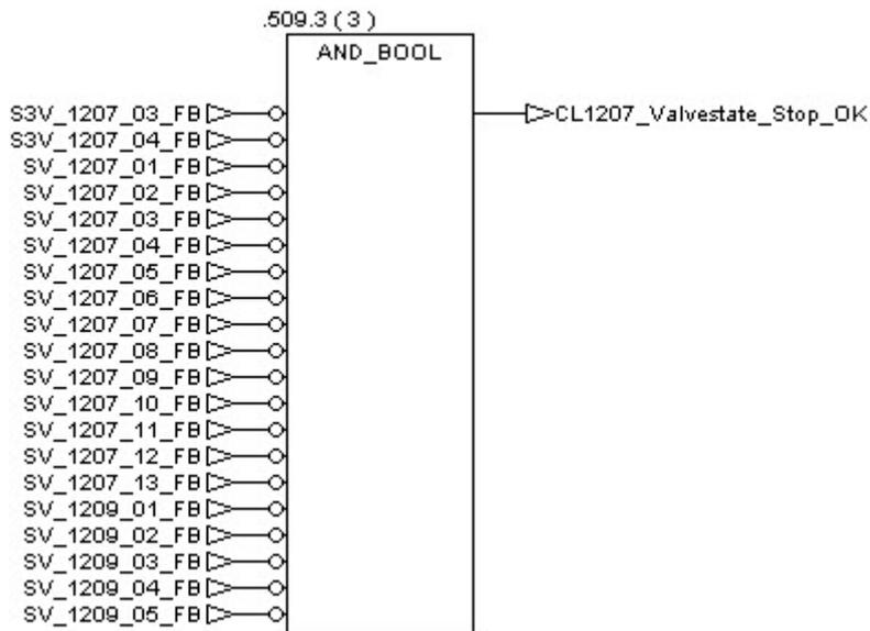
Once the valve status is OK, cleaning pumps are reset.
