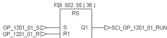
The tag “SCI\_GP\_1201\_01\_RUN” is the condition to start or stop the pump if no error is detected.
