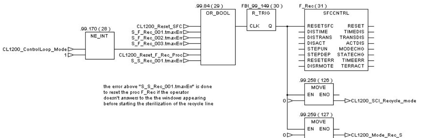
If a time error occurs during the execution of the procedure, SFC\_CNTRL reset the procedure, the tag linked to the procedure.
