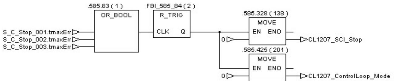
In Parallel, the procedure named “CL1207\_ RESET\_PROC” is started. This procedure, detailed further on, triggers a general reset (CIP procedures and equipments) to ensure the default status of all the Cleaning function when automatic mode is re-started.
