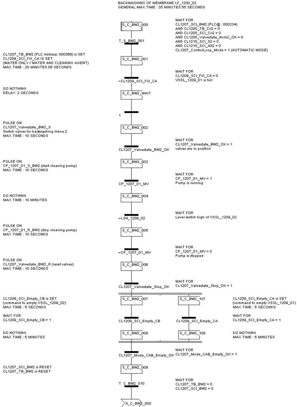
Figure 130: PLC procedure: C\_BW2
