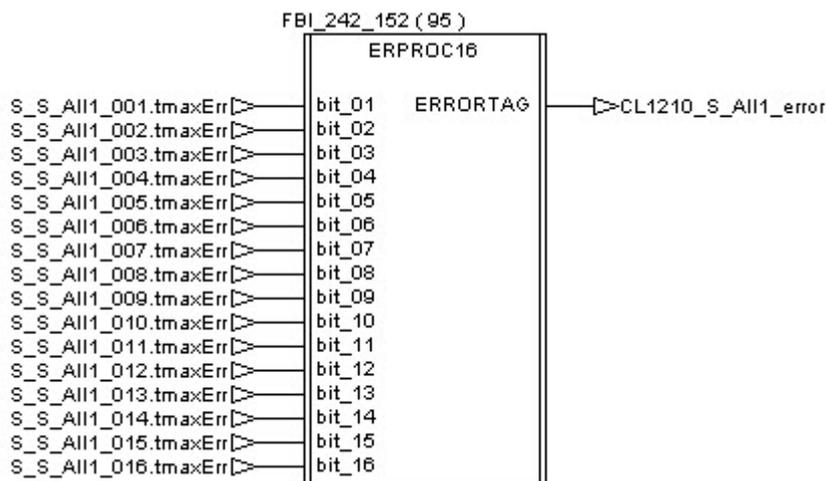
If an error is detected during the execution of the procedure, the tag “CL1210\_S\_ALL1\_error\_Stop” receives a pulse and then the Sterilization Unit is stopped thanks to the procedure “S\_Stop”.
