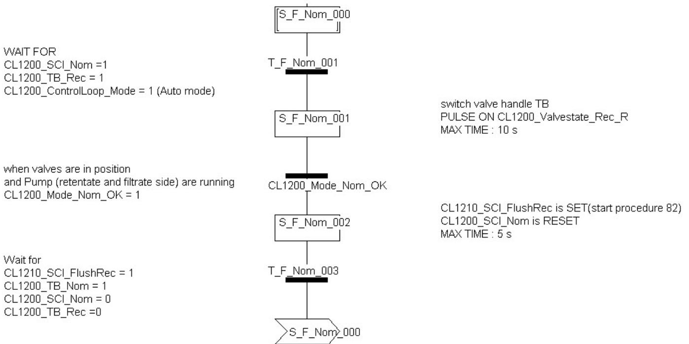
Figure 122: PLC procedure: F\_Nom
