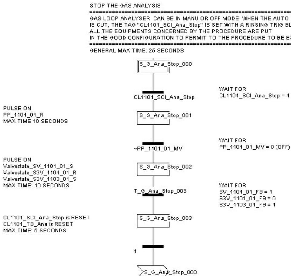
Figure 109: PLC procedure: G\_Ana\_Stop
