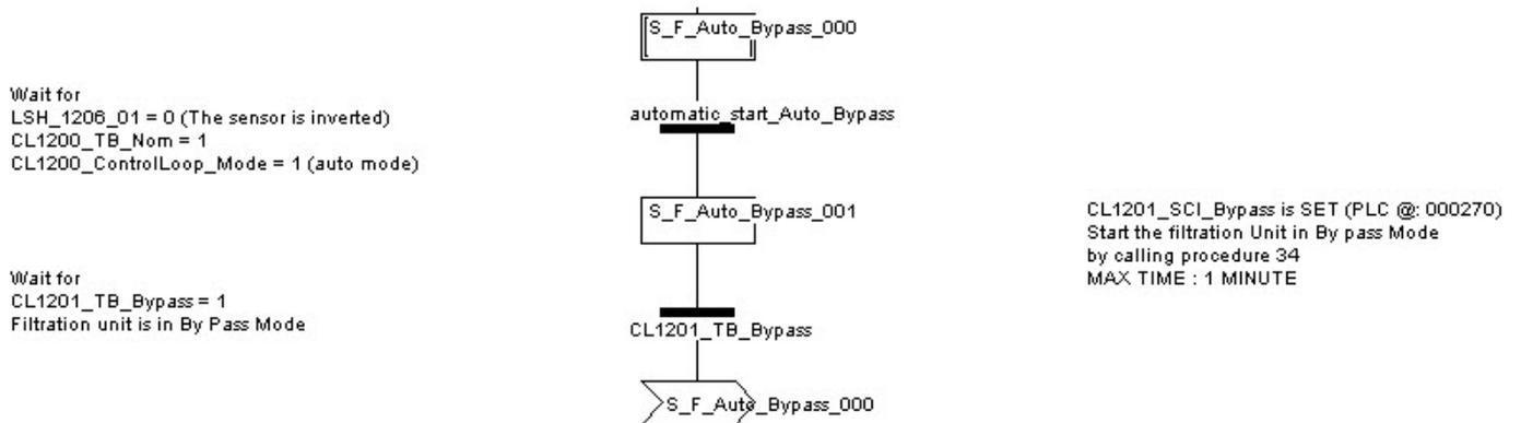
Figure 154: PLC procedure: F\_Auto\_Bypass
