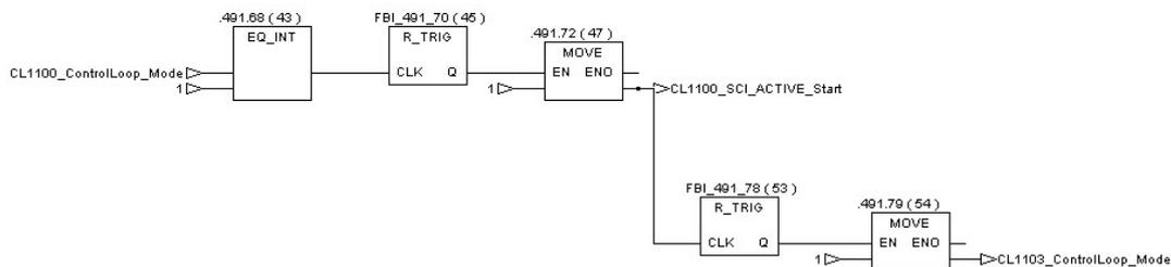
When the Control Loop mode is configured to OFF or Manual mode, the procedure “G\_Active\_Loop” and all equipments linked are stopped.
