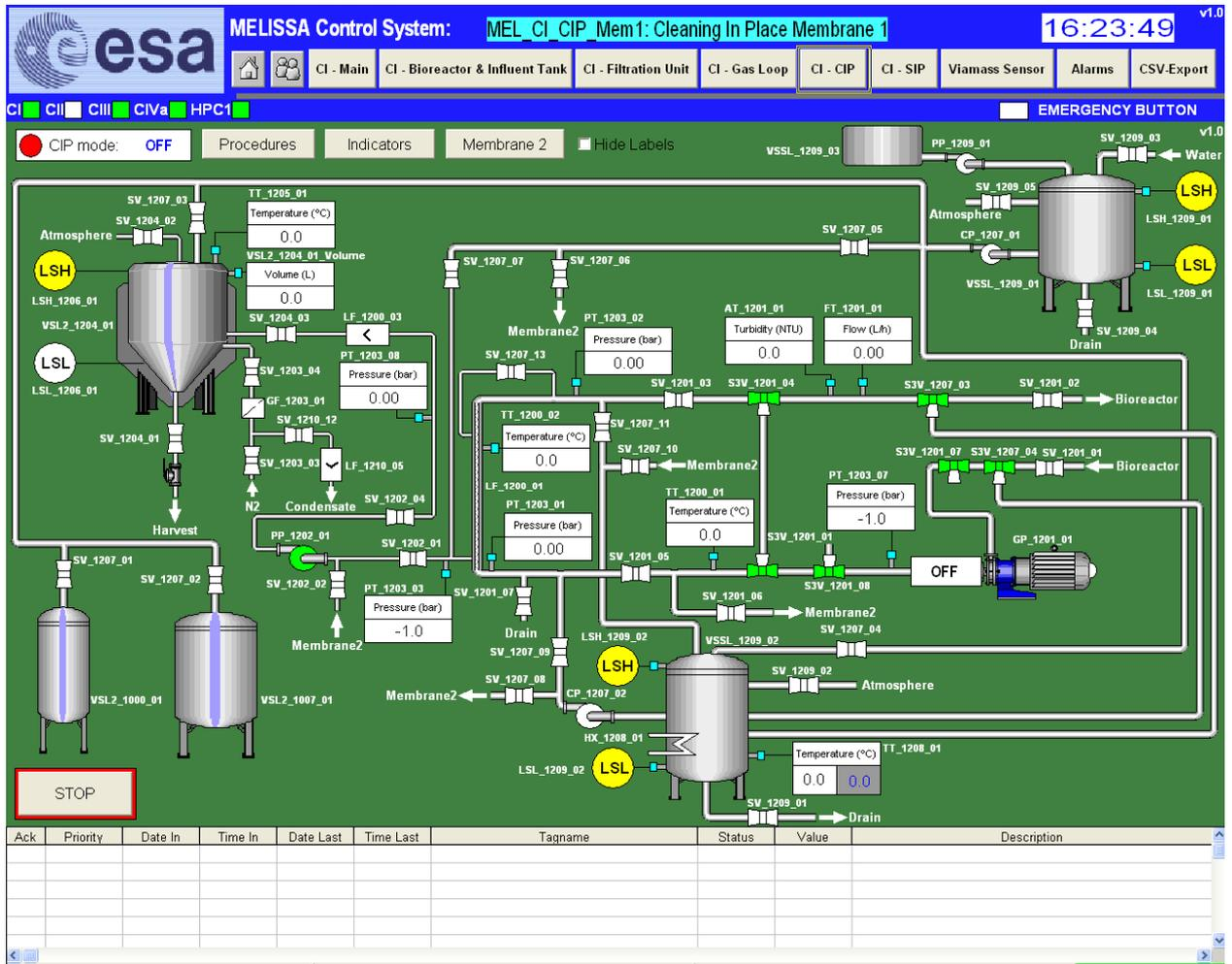
Figure 6-26: Main objects in Membrane 1 CIP screen
