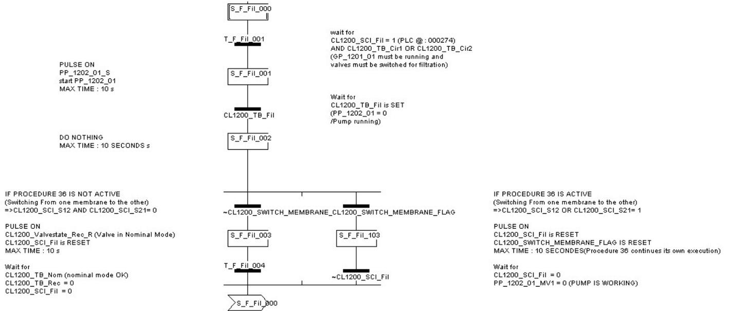
Figure 117: PLC procedure: F\_Fil
