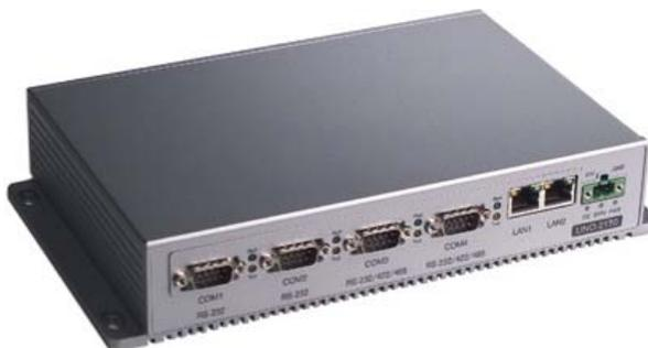
Embedded pc is the interface between biomass sensor and PLC. The current version takes data from biomass sensor box (bioimpedance value) and sends it to the plc through serial modbus. In future version, it will estimate the biomass present in the bioreactor. For further information see NTE-VSS-HB-017 and NTE-VSS-HB-018 documents.
