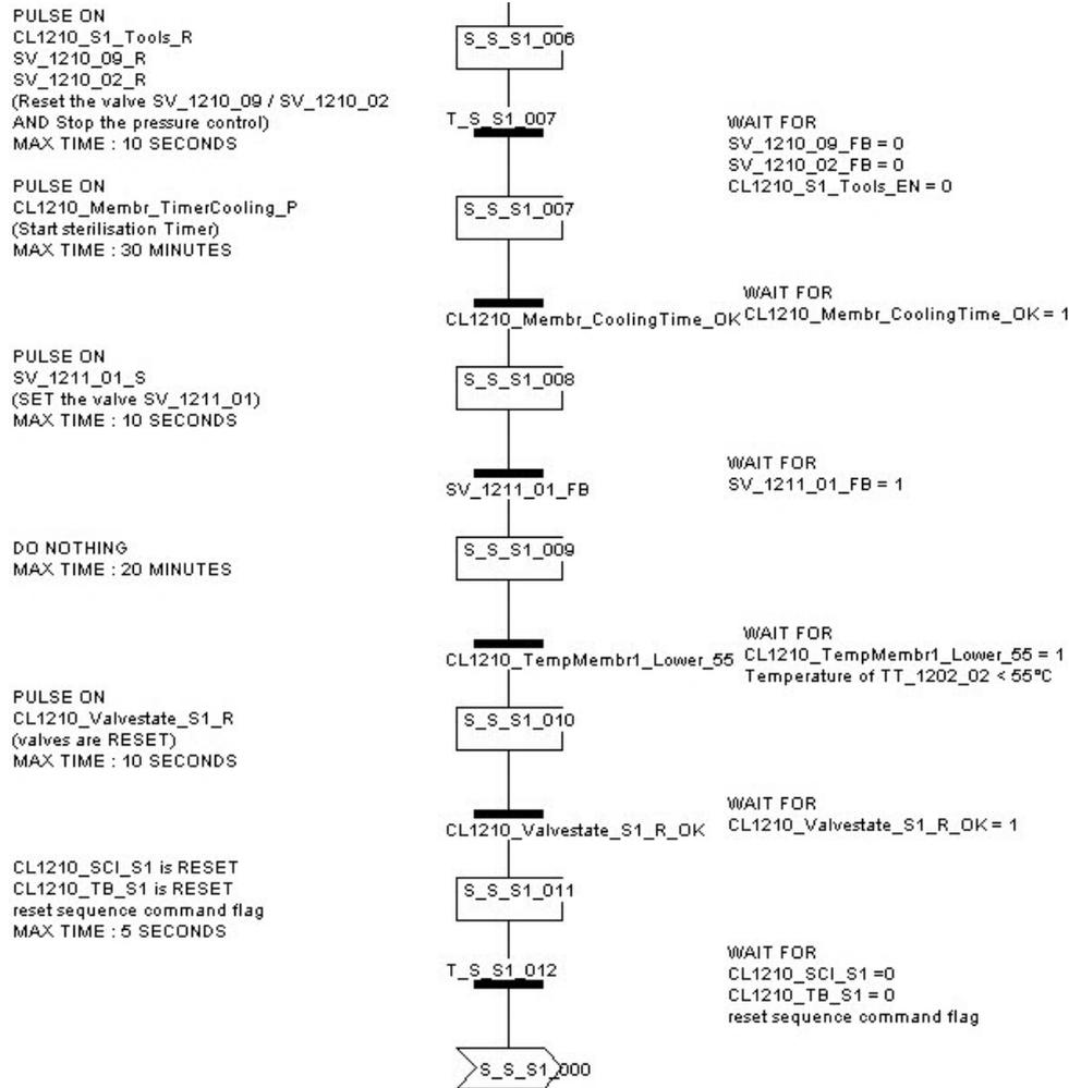
Figure 147: PLC procedure: S\_S1
