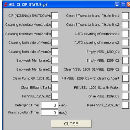
Figure 6-29: Indicators of the CIP procedures
