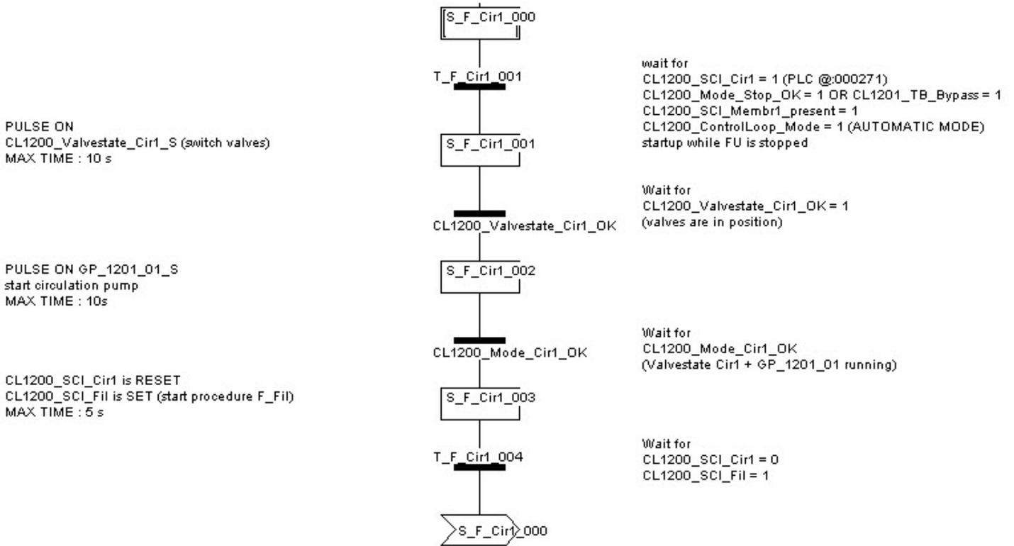
Figure 115: PLC procedure: F\_Cir1
