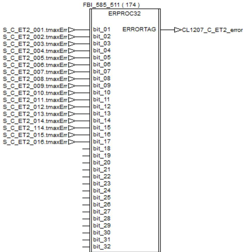
If an error is detected during the execution of the procedure, the tag “CL1207\_C\_ET2\_error\_Stop” receives a pulse and then the Cleaning Unit is stopped thanks to the procedure “C\_Stop”.
