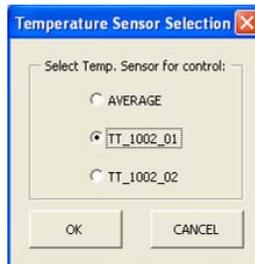
Figure 6-9: Influent tank temperature probe selection
