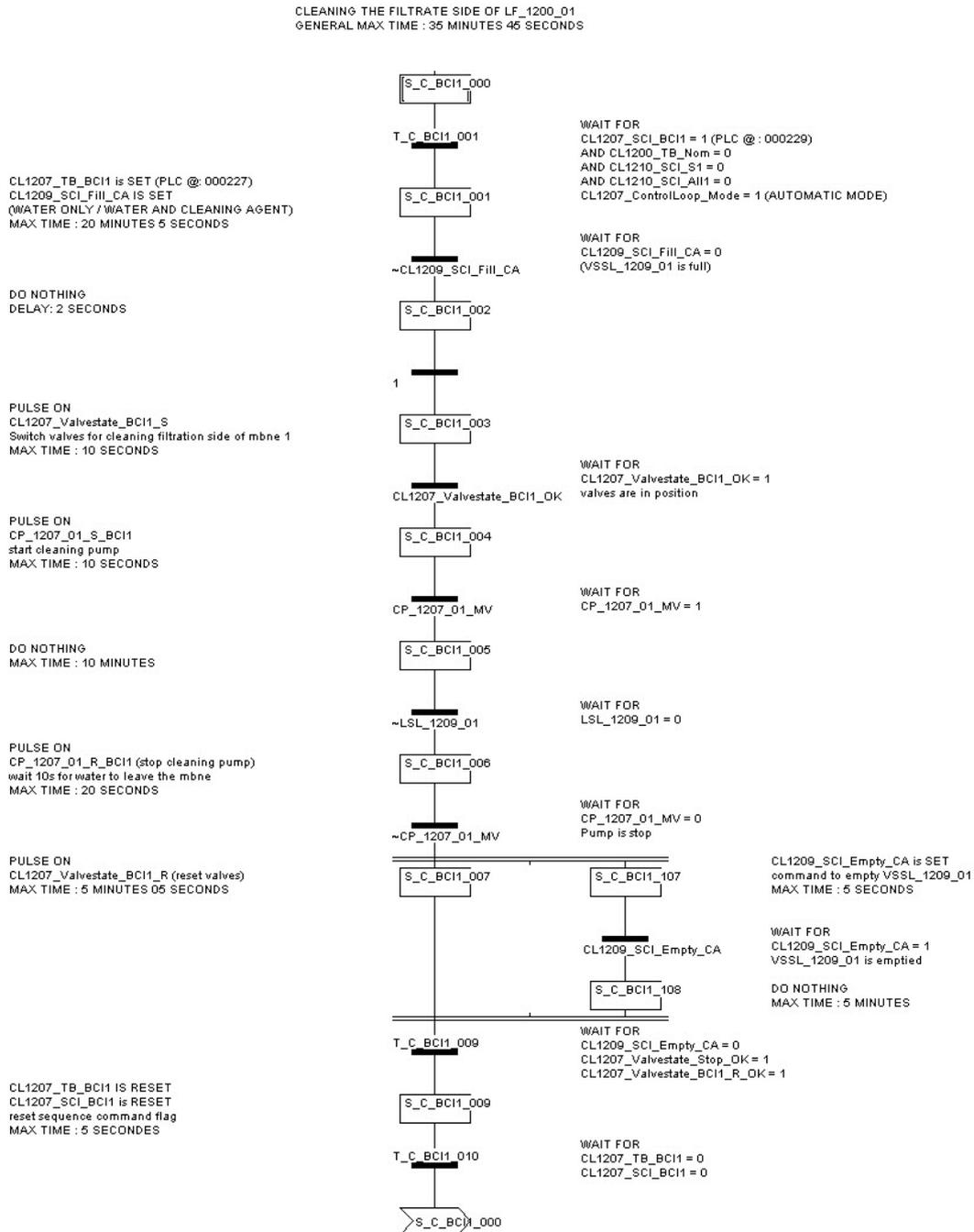
Figure 127: PLC procedure: C\_BCI1
