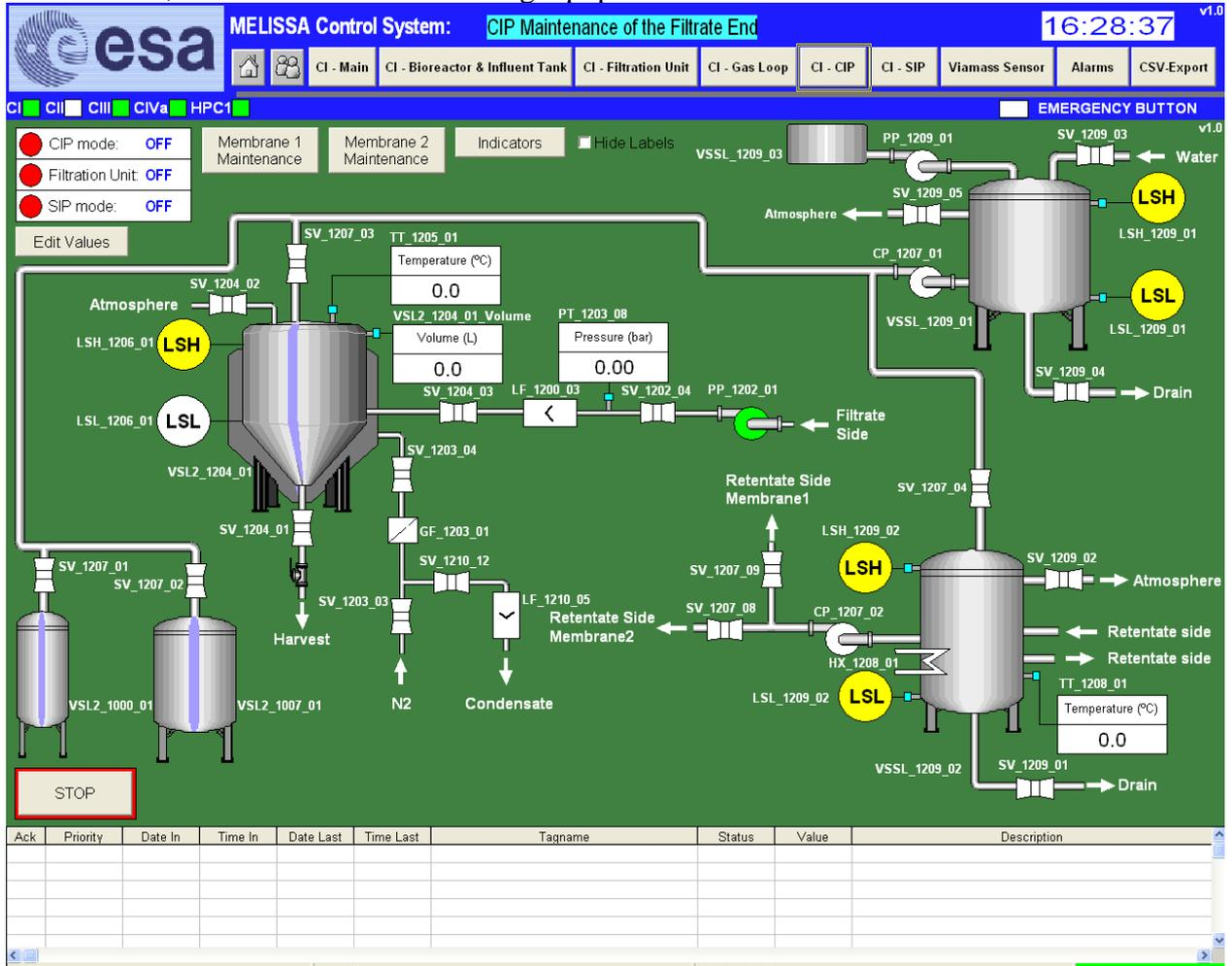
Figure 6-31: Main objects of the CIP Maintenance screen (Filtrate side)
