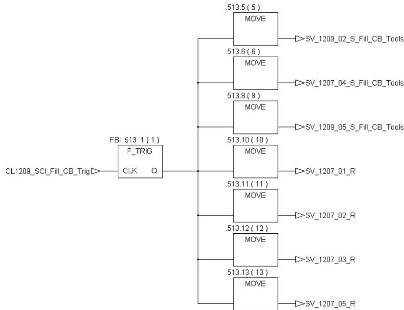
When the VSSL\_1209\_02 is full, the level switch High LSH\_1209\_02 is reset (inverted logic) and a pulse is sent to close the atmospheric valve of both cleaning vessels SV\_1209\_02 and SV\_1209\_05 and the entrance valve of VSSL\_1209\_02 (SV\_1207\_04).
