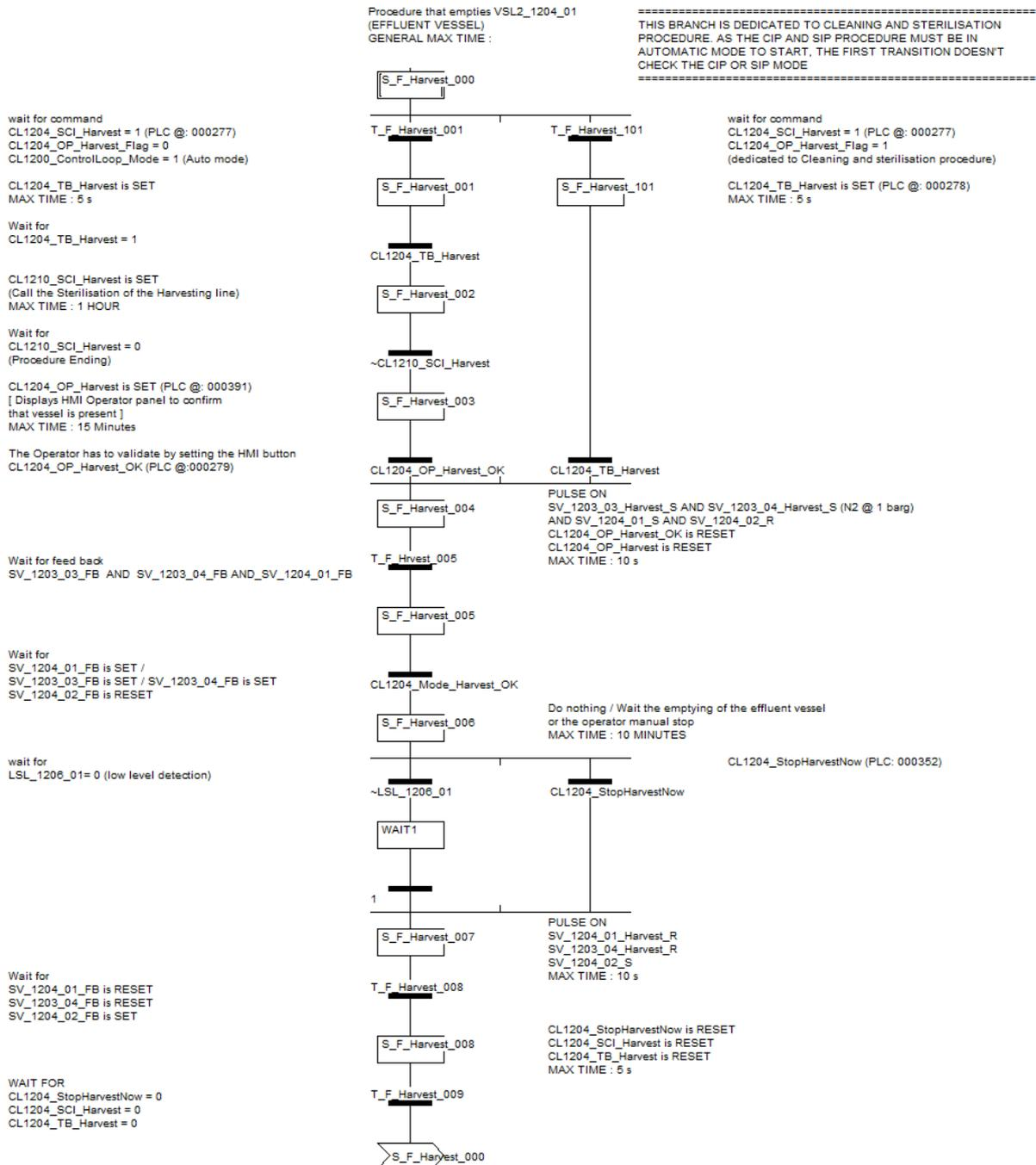
Figure 123: PLC procedure: F\_Harvest
