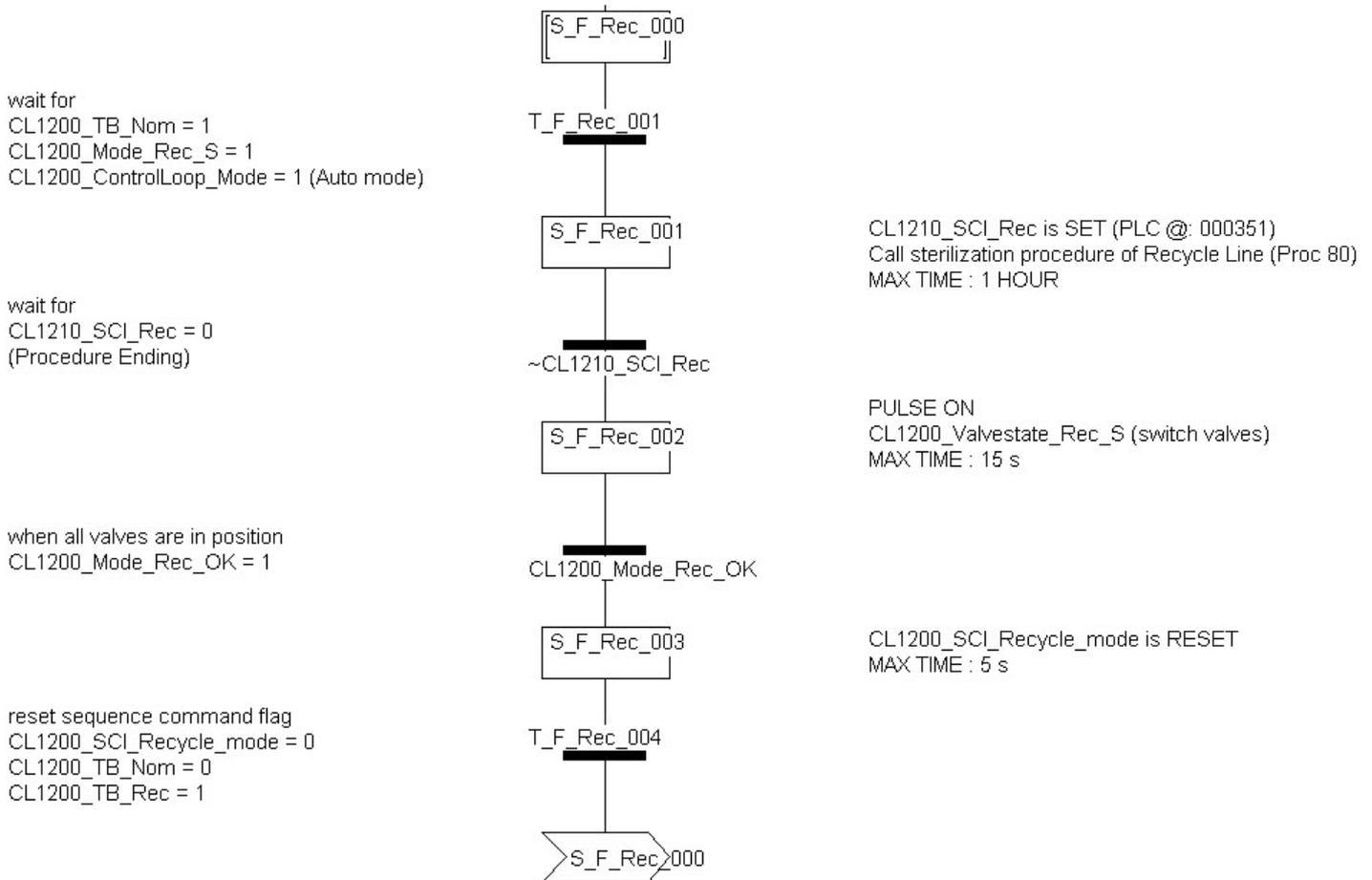
Figure 121: PLC procedure: F\_Rec
