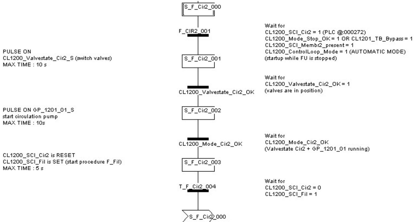
Figure 116: PLC procedure: F\_Cir2
