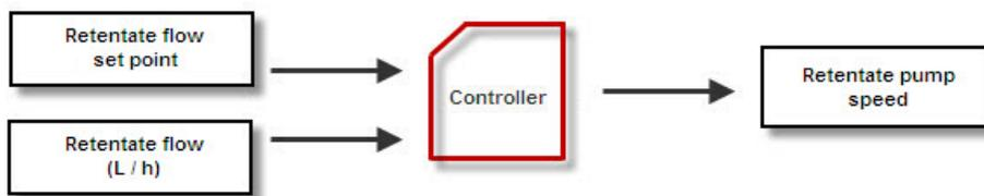
The retentate flow is controlled by a PI controller. Depending on the set point, the controller will adjust the retentate flow thanks to the speed of the pump GP\_1201\_01.
