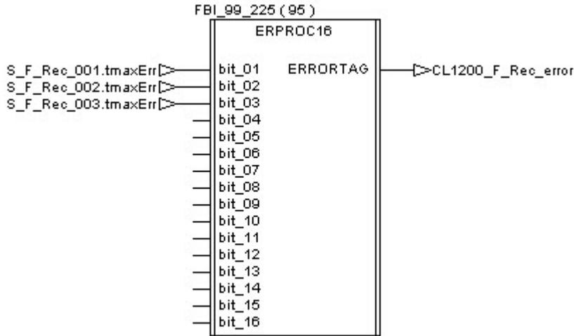
If an error is detected during the execution of the procedure, the tag “CL1200\_F\_Rec\_error\_Stop” receives a pulse and then the Filtration Unit is stopped thanks to the procedure “F\_Stop”.
