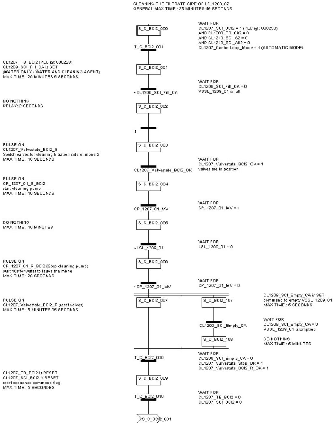
Figure 128: PLC procedure: C\_BCI2
