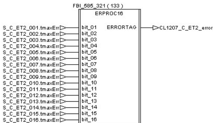
Internally, each step represents a bit of a word (16 bits). When an error appears, the “R\_TRIG” block sends a pulse and activates for one PLC Cycle a “MOVE block”. At the same time, the same bit is recorded as a UDINT (Unsigned integer variable: 32 bits) in the tag situated at the output of the “ERPROC16” block. As the output of the block is no more activated after the pulse, the error is frozen. The reset of this error variable is done when the procedure is re-started.
