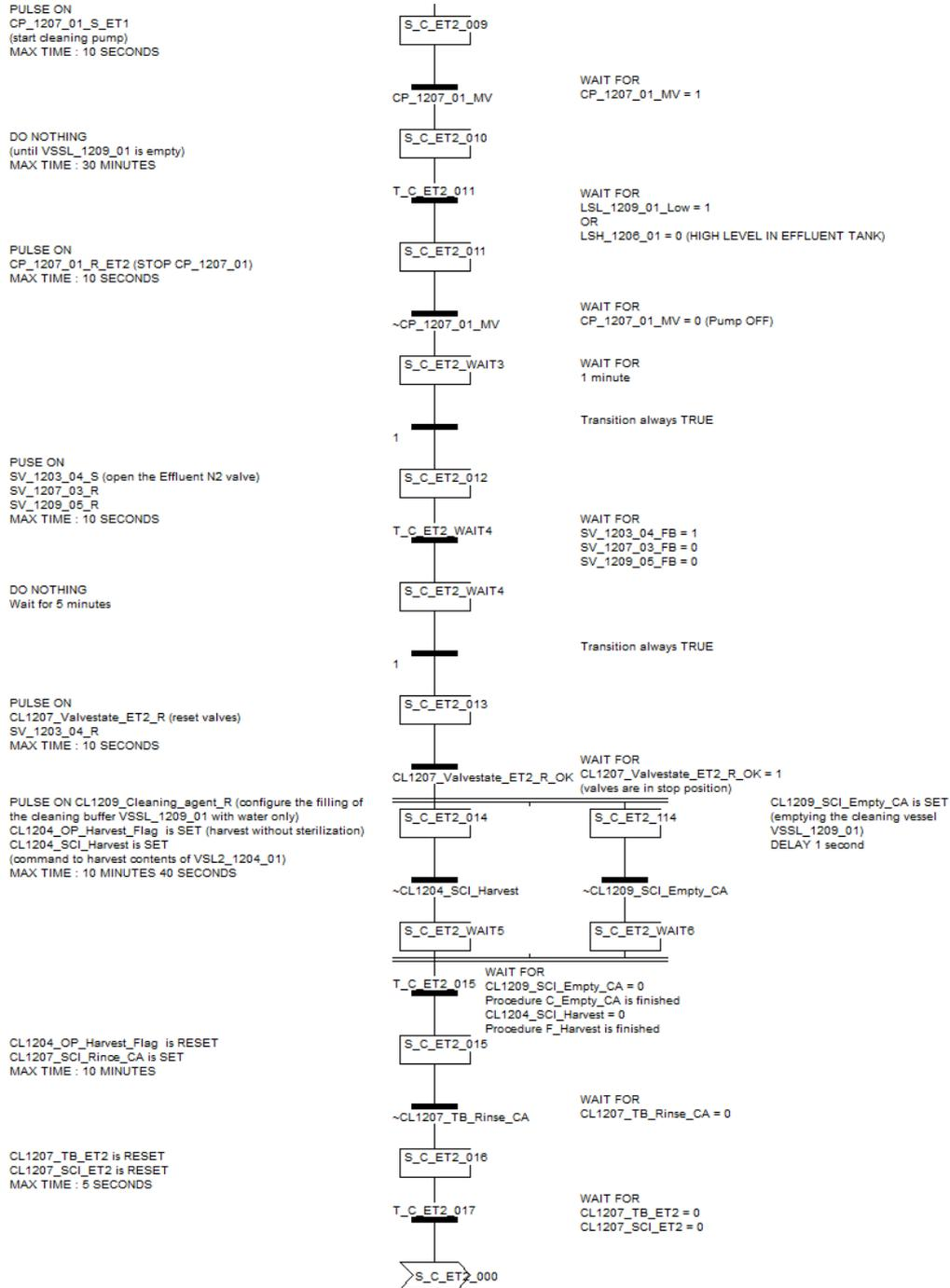
Figure 134: PLC procedure: C\_ET2
