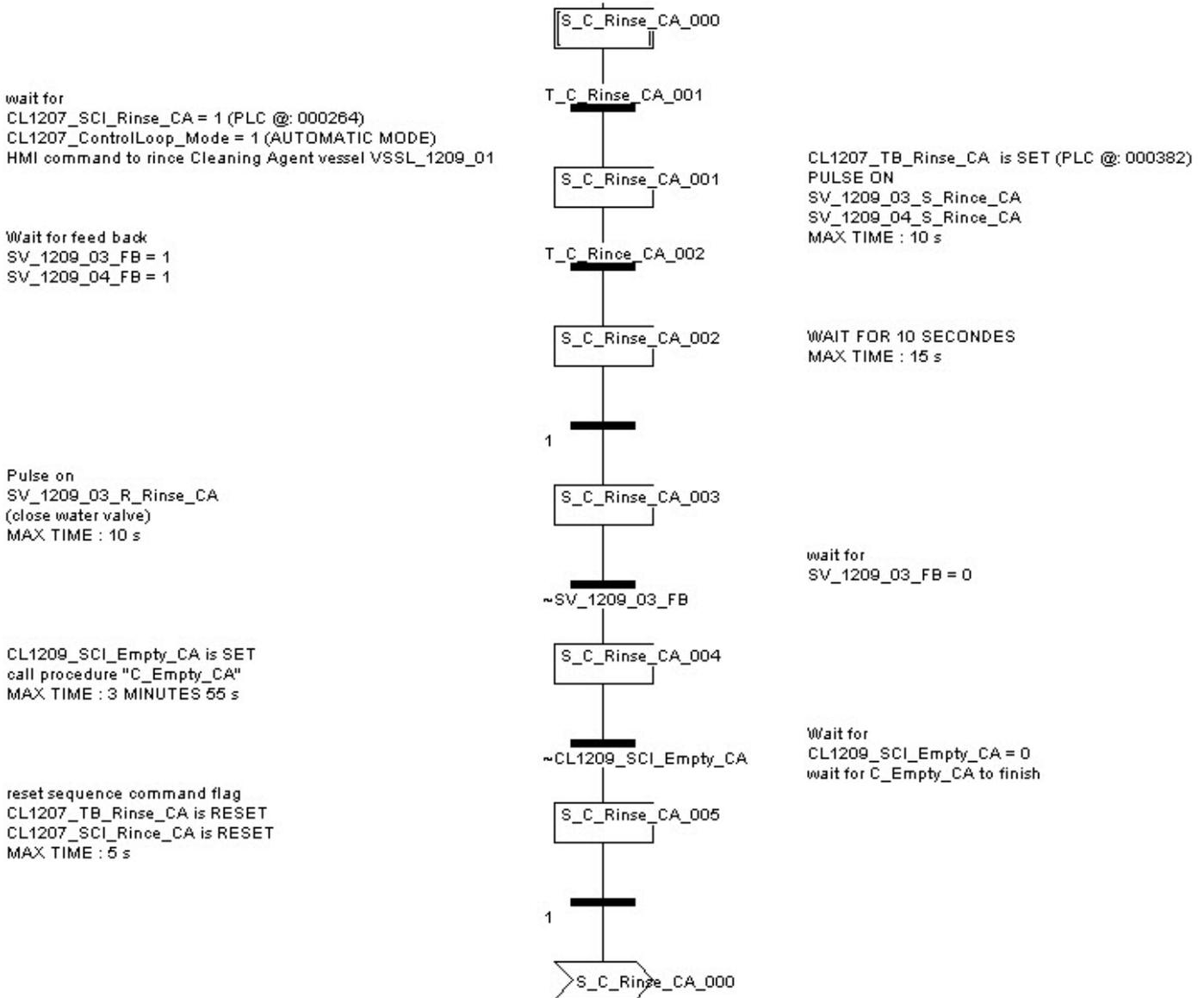
Figure 144: PLC procedure: C\_Rinse\_CA
