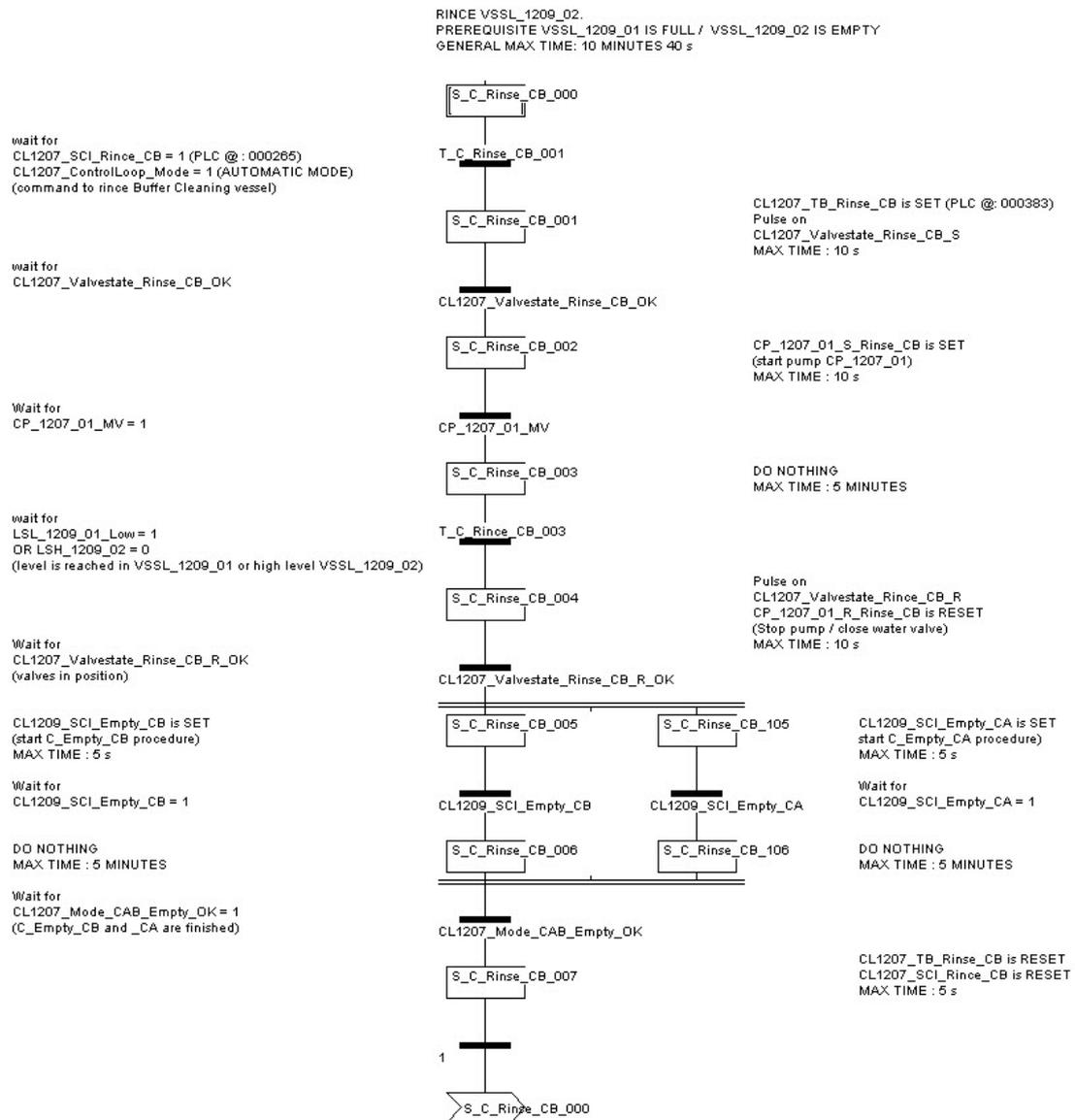
Figure 145: PLC procedure: C\_Rinse\_CB
