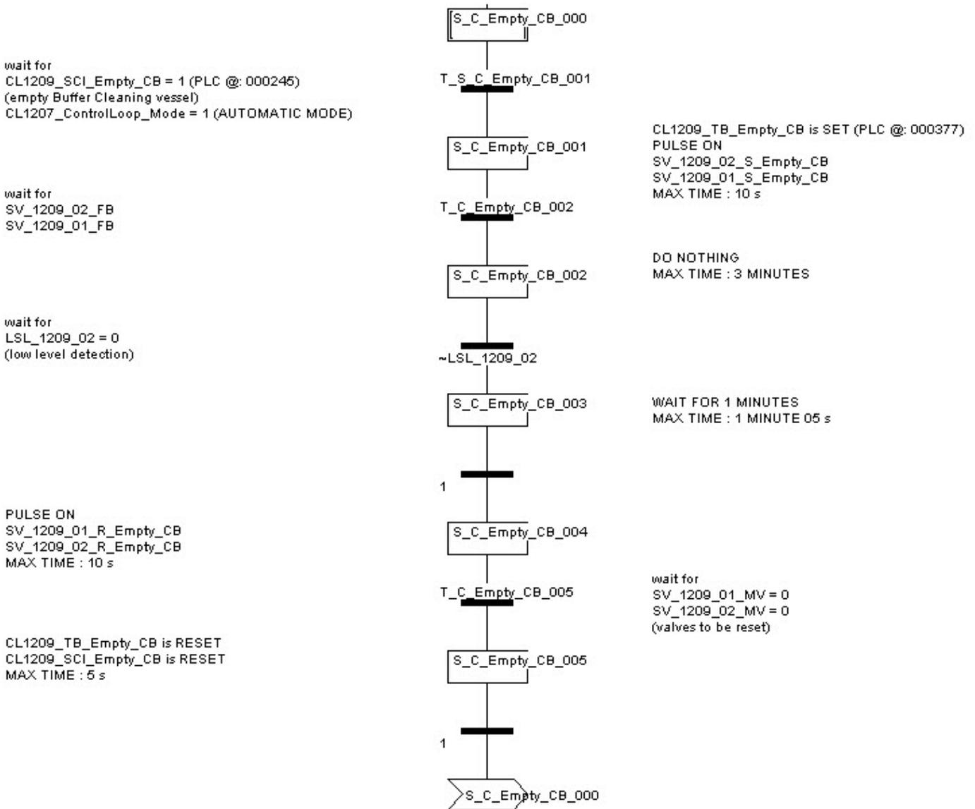
Figure 139: PLC procedure: C\_Empty\_CB
