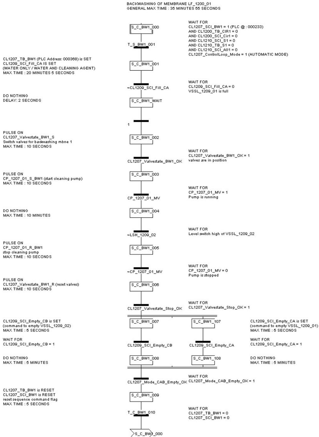
Figure 129: PLC procedure: C\_BW1
