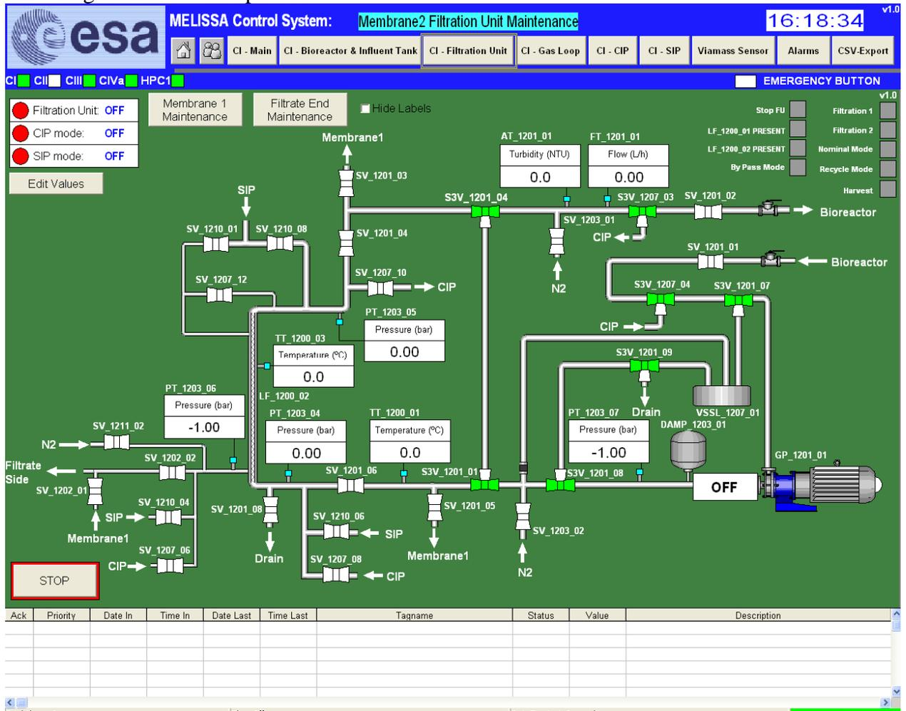
Figure 6-24: Main objects of the Filtration Unit Maintenance screen (Membrane 2 side)
