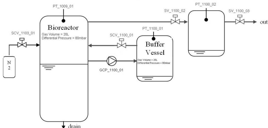
The gas loop pressure control represents the Active Gas loop. A procedure named “G\_Active\_Loop” which manages the active gas loop is detailed in the chapter “User Manual Procedures”.
