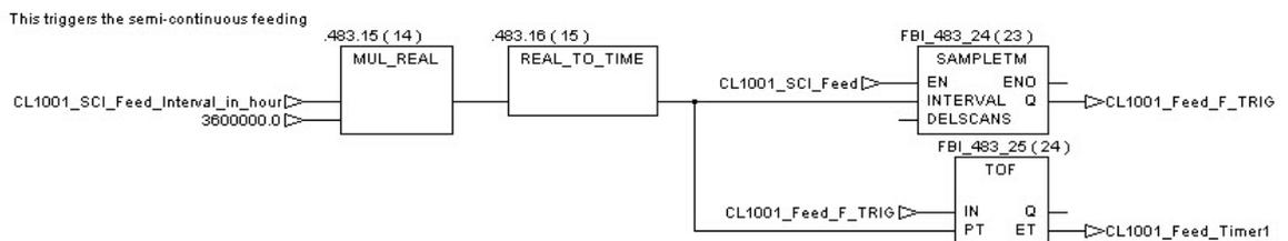
Once set, depending on the selected mode (Timer / Volume), the variable “CL1001\_Feed” is set to feed the bioreactor by the valve S3V\_1001\_01 as follow.
