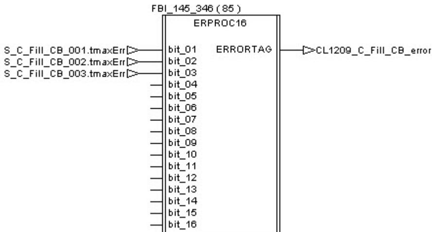
If an error is detected during the execution of the procedure, the tag “CL1207\_C\_FILL\_CB\_error\_Stop” receives a pulse and then the Cleaning Unit is stopped thanks to the procedure “C\_Stop”.
