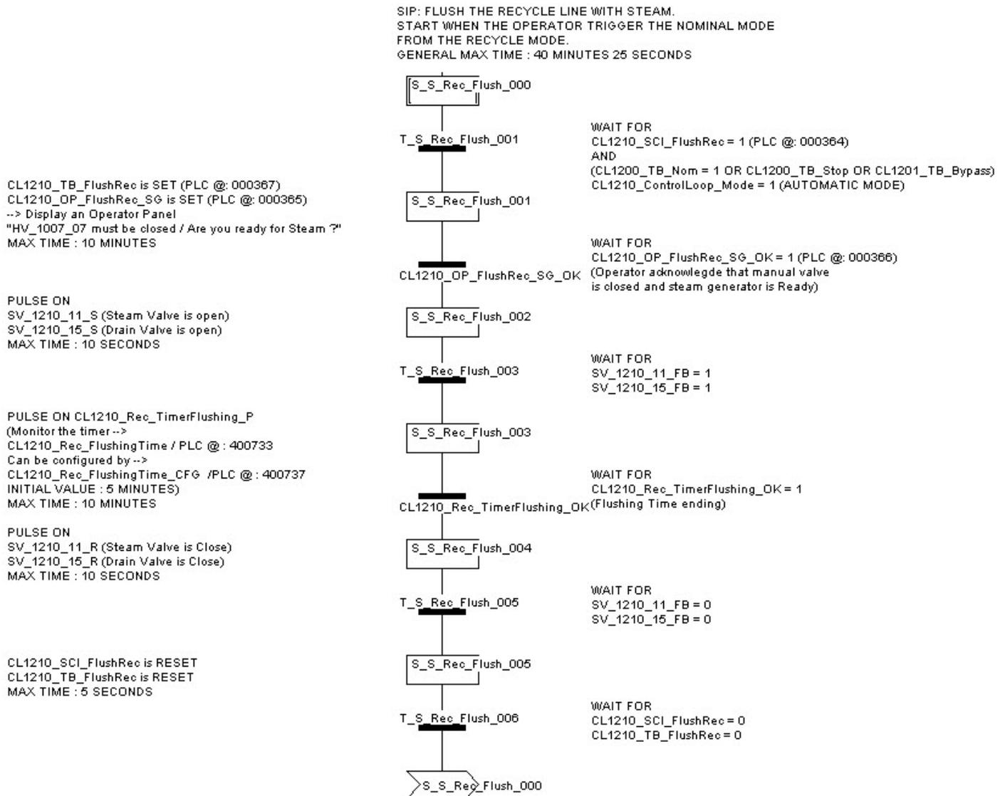
Figure 153: PLC procedure: S\_Rec\_Flush
