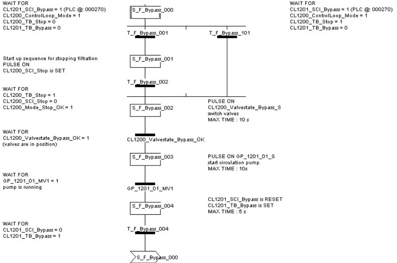
Figure 114: PLC procedure: F\_Bypass
