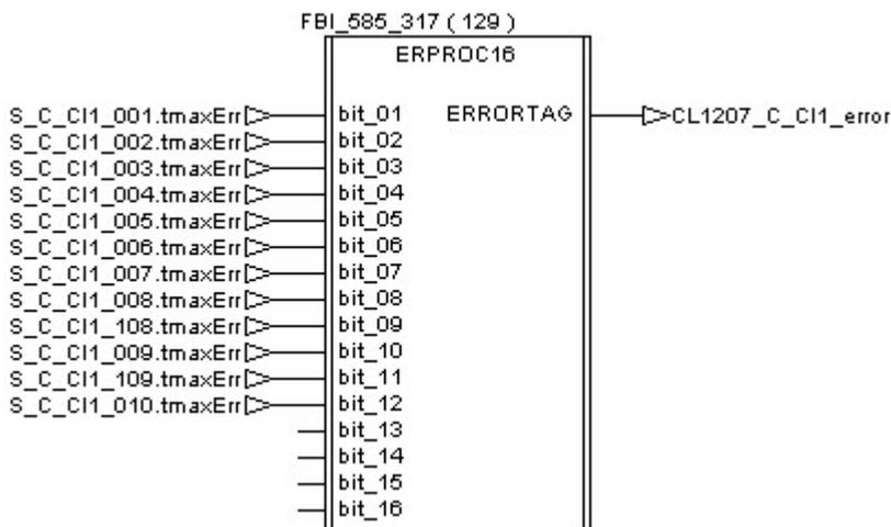
If an error is detected during the execution of the procedure, the tag “CL1207\_C\_C11\_error\_Stop” receives a pulse and then the Cleaning Unit is stopped thanks to the procedure “C\_Stop”.
