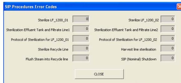
Figure 6-39: Error Codes of the sterilization in place procedures
