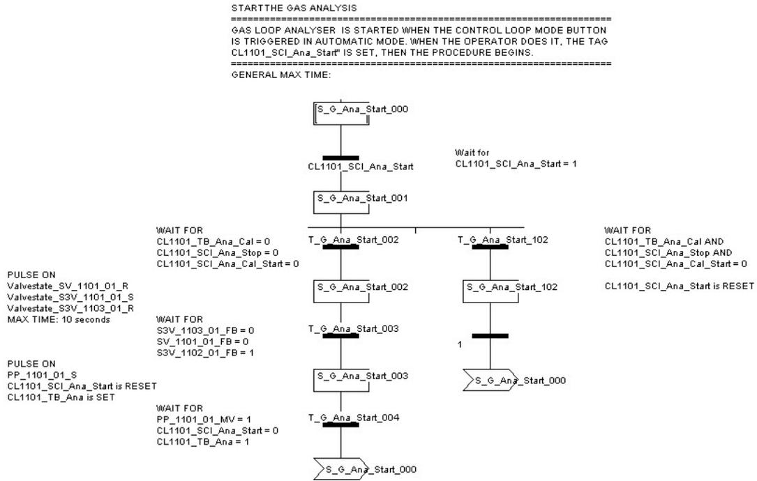
Figure 110: PLC procedure: G\_Ana\_Start
