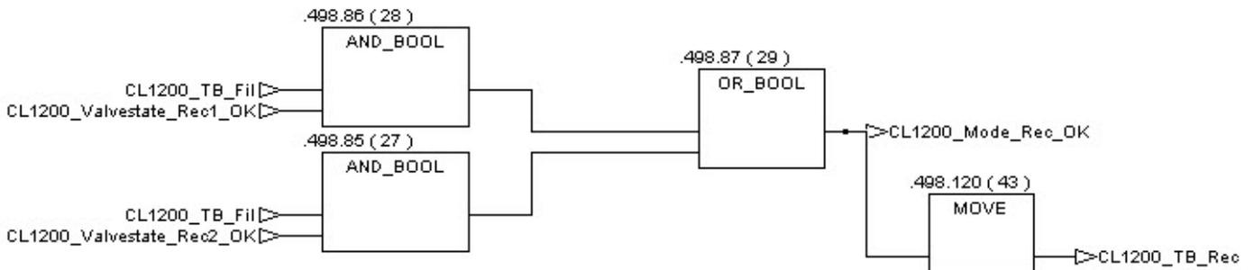
Figure 120: PLC Block: F\_MODE\_REC
