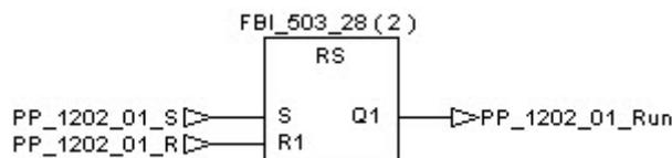
The tag “PP\_1202\_01\_RUN” is the condition to start or stop the pump if the effluent tank level switch high is not set.
