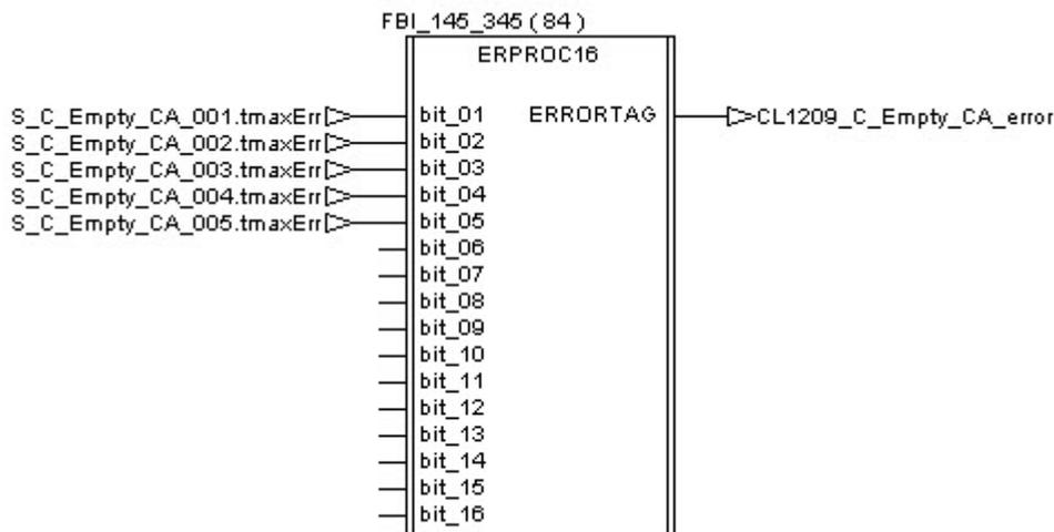
If an error is detected during the execution of the procedure, the tag “CL1207\_C\_EMPTY\_CA\_error\_Stop” receives a pulse and then the Cleaning Unit is stopped thanks to the procedure “C\_Stop”.
