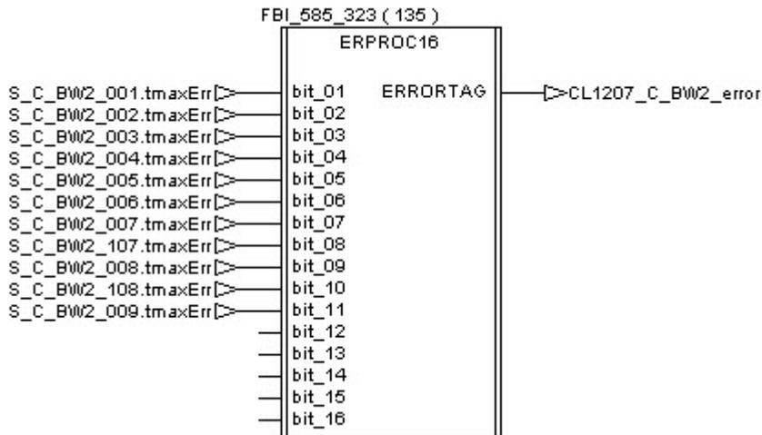
If an error is detected during the execution of the procedure, the tag “CL1207\_C\_BW2\_error\_Stop” receives a pulse and then the Cleaning Unit is stopped thanks to the procedure “C\_Stop”.
