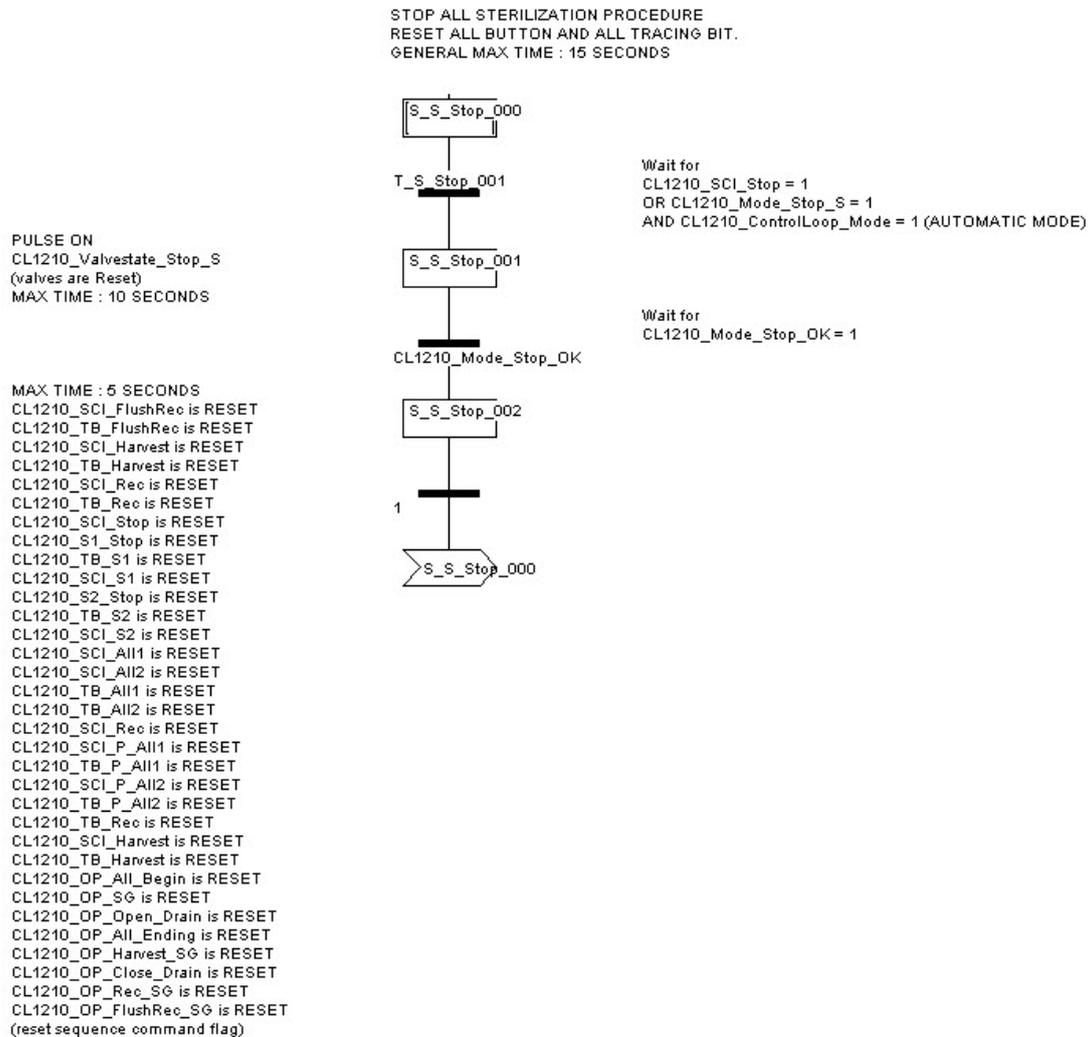
Figure 146: PLC procedure: S\_Stop
