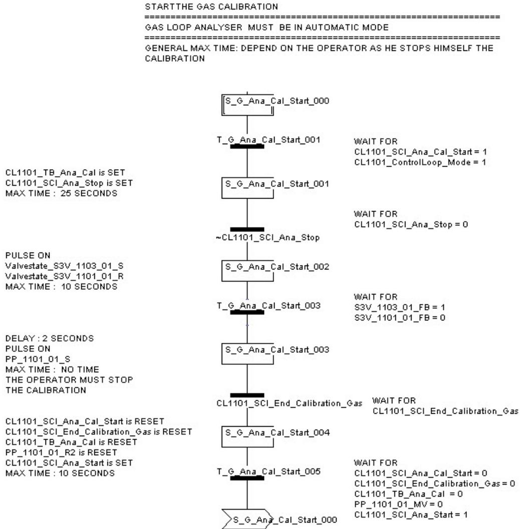
Figure 111: PLC procedure: G\_Ana\_Cal\_Start
