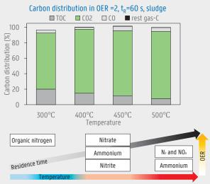
Some carbon was kept in solid products in low temperature and low OER cases. Carbon dioxide and carbon monoxide could be found in most gas effluent. Longer residence time could increase carbon recovery but at low rate. Organic nitrogen was mostly converted to ammonia with increasing temperature and prolonged residence time, however, along with high conversion to N<sub>2</sub> and NO.
