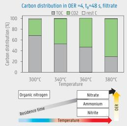
No solids were found in final products, carbon dioxide was the only carbon gas. Carbon recovery of filtrate was lower compared sludge oxidation. Ammonium was the main nitrogen product and no nitrogen was lost in gas phase. Nitrate was slightly converted in given conditions.
